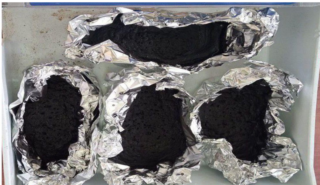
Figure 8: Concentrated coals after flotation in the aluminum foil paper of the study area
