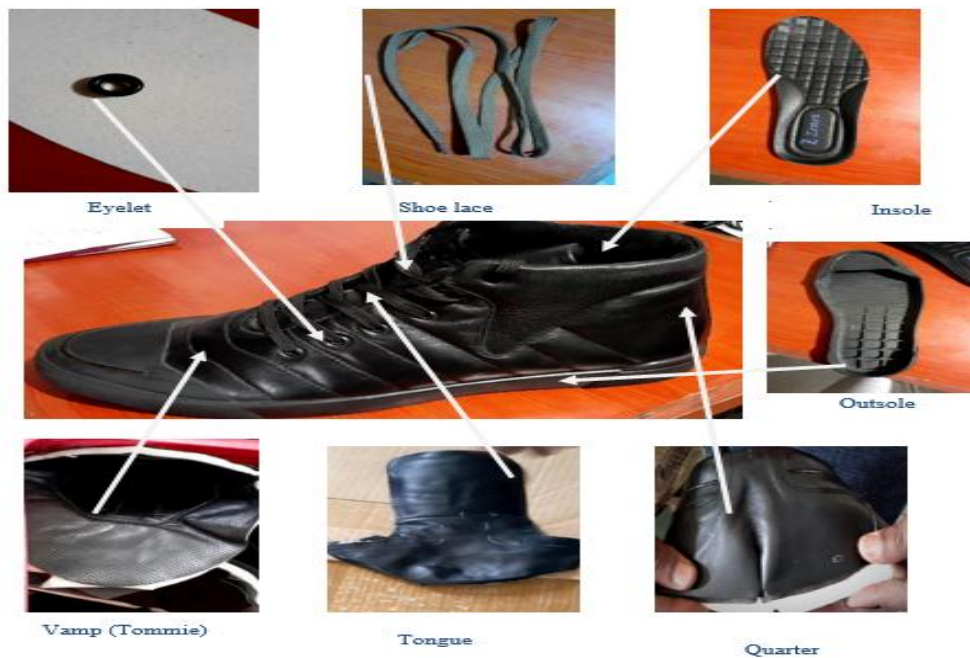
Figure 4. 6: Major Components of Model 23 Shoe (Author)
