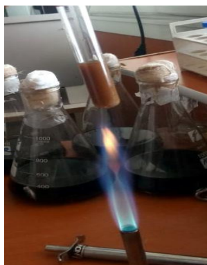
Figure 4: 1 Result of benedict test of hydrolyze sugar cane bagasse
