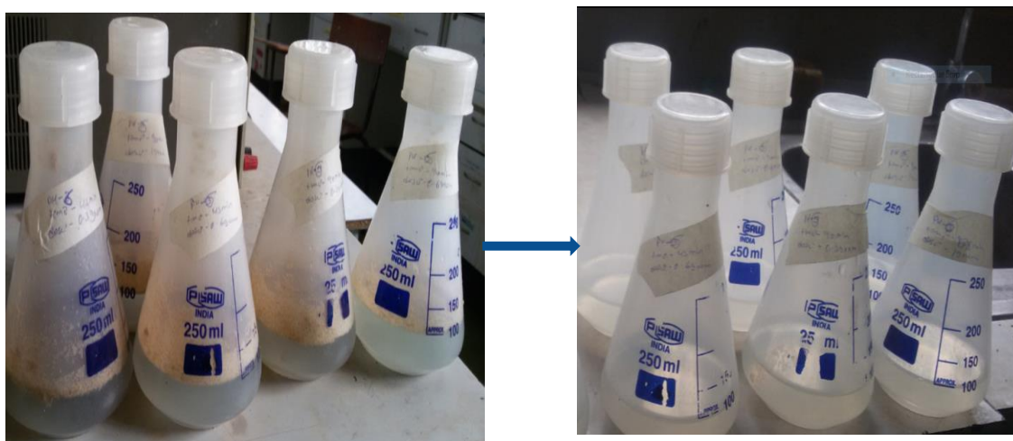
Figure 3.4: Batch adsorption set up (A) Samples before Adsorption and (B) Samples after adsorption
