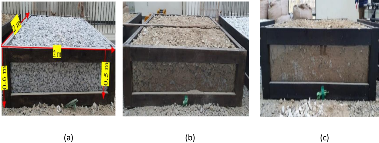
Figure 5.2 fouling ballast condition (a) Box 1, (b) Box 2 and (c) Box 3. [42]
