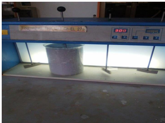
Figure C- 2. Mixing of pulp slurry
