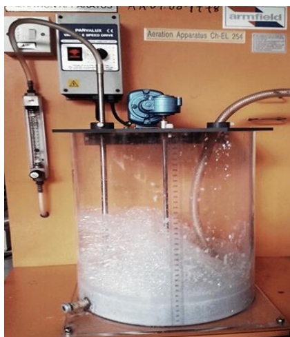
Figure 3.1. Aeration apparatus of flotation process
