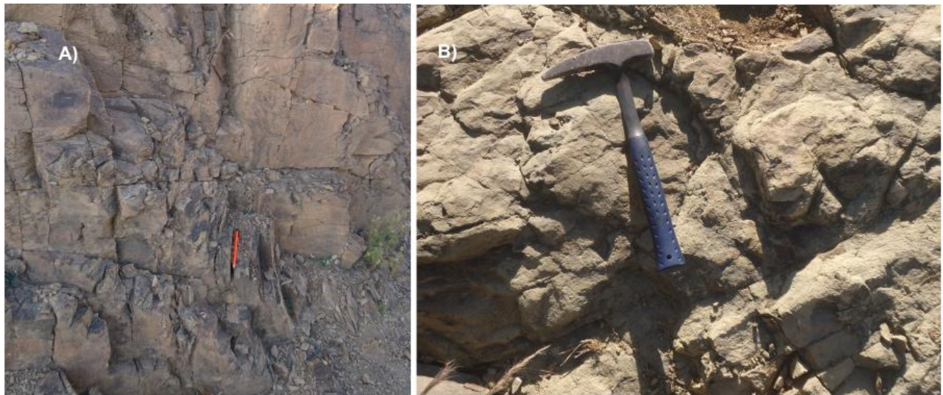
Figure 3.15. Outcrop photo of metatuff unit. A) It is foliated, moderately compacted and cross cut by a systematically aligned joint and this photo is taken facing to NW (0495770 E:1553076 N). B) This unit is more compacted having light grey color and the photo is taken facing to N direction (0495367E:1553060N).
