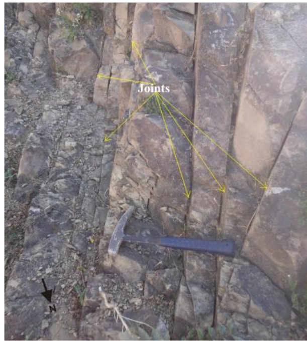
Figure 4.14. Systematic joint sets crosscutting the compacted metatuff units (0495770 E: 1553076 N).
