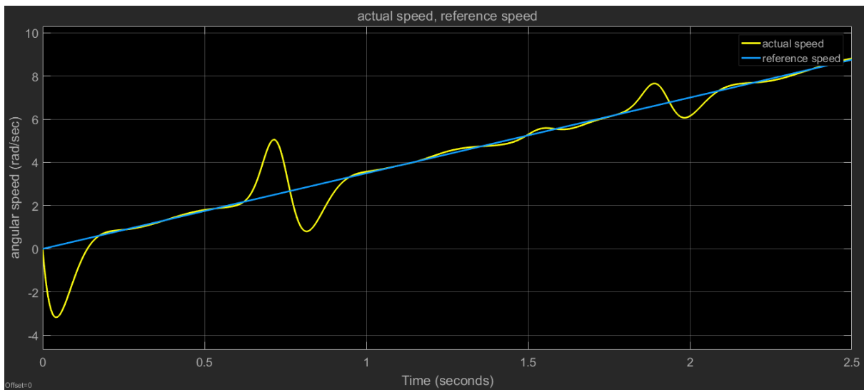
Figure 4.7 Speed Response of PI Controller with Adhesion Torque Load
