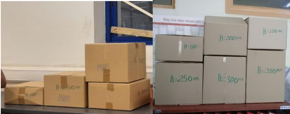
Figure 3.13: Samples of corrugated box at height of h=150/200/250/300/350 mm.
