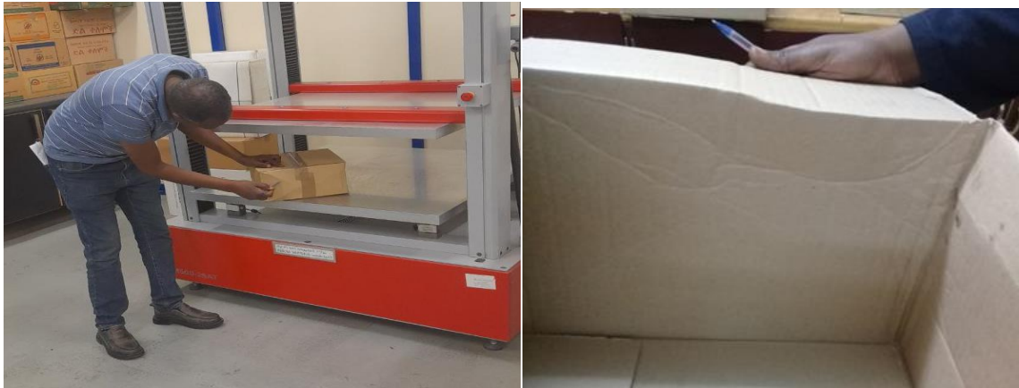
Figure 3.14: BCT of computerized electronic testing machine at unlimited packaging plc.
