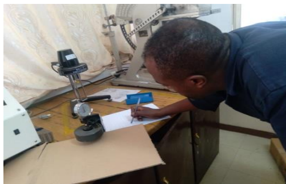
Figure 3. 3 :Measuring board and paper thicknesses.
