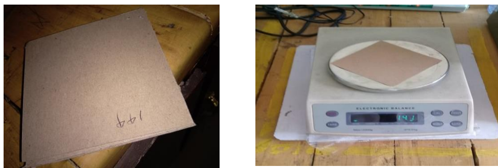
Figure 3. 2 Measuring paper grammage
