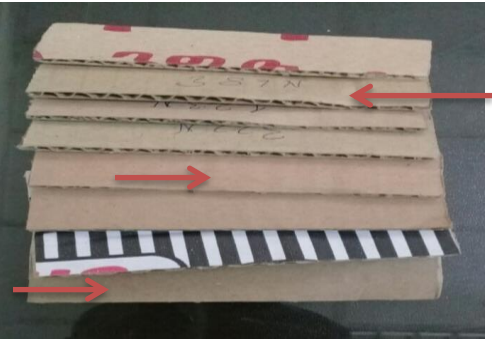
b, failure under compression
