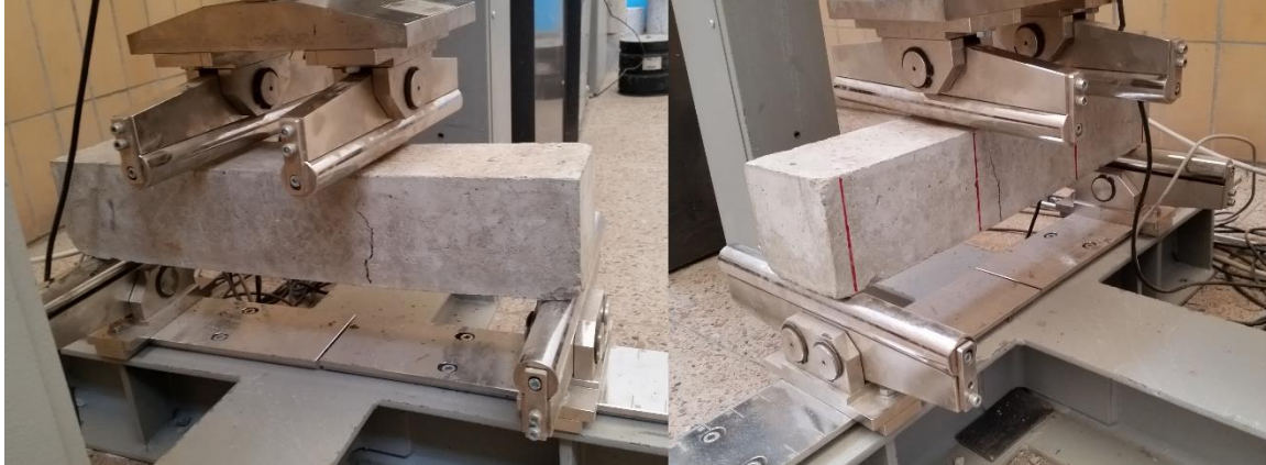
Figure 5.2. A concrete beam after completion of flexural strength test.
