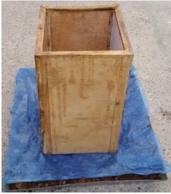
Figure 4.3. A rectangular formwork (greased) prepared for casting sample concrete for temperature test.
