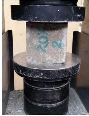
Figure 5.4. A concrete cube under compressive strength test.
