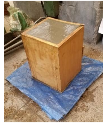
Figure 4.4. Sample concrete (right after casting) prepared for temperature test.
