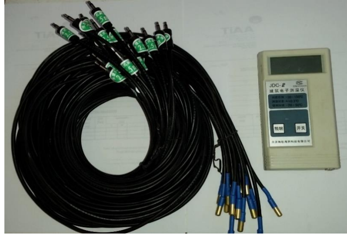
Figure 5.6. Thermocouples and temperature reader that was used to measure temperature
