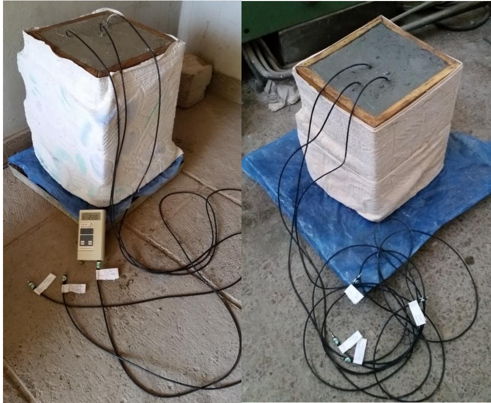
Figure 4.5. Temperature measurement of concrete samples with different percentages of bagasse ash
