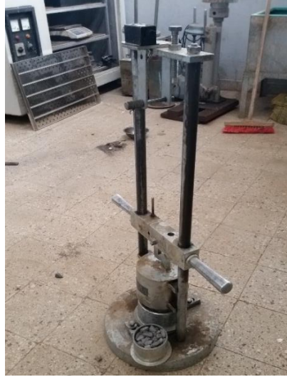
Figure 3.3. Sample aggregate prepared for conducting AIV test and an apparatus used for measuring AIV
