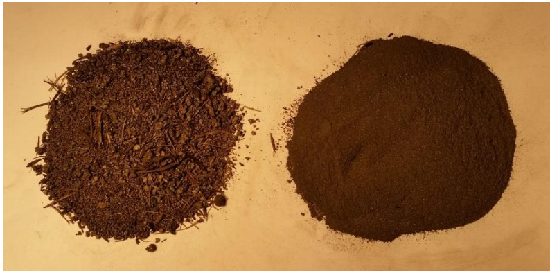
Figure 3.9. Bagasse ash before (left) and after (right) sieving (with 300 \mu m sieve)
