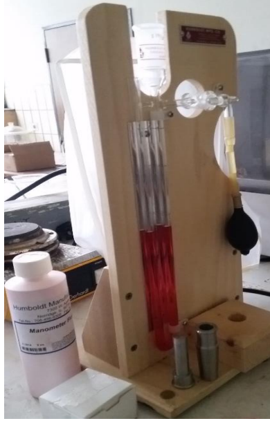
Figure 3.6. Blaine air permeability apparatus used to test fineness of cement and bagasse ash
