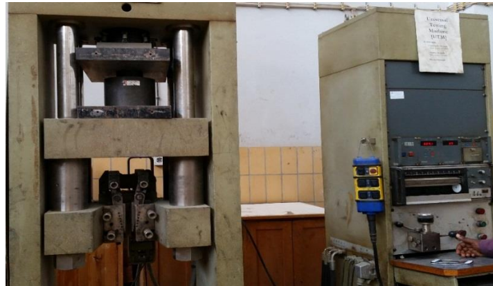
Figure 3.2. Sample aggregate under ACV test
