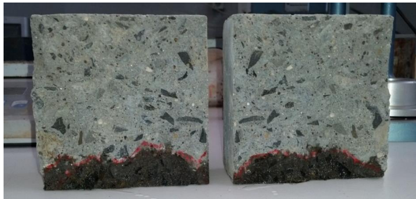
Figure 5.11. Concrete cube sample split after passing water penetration test.
