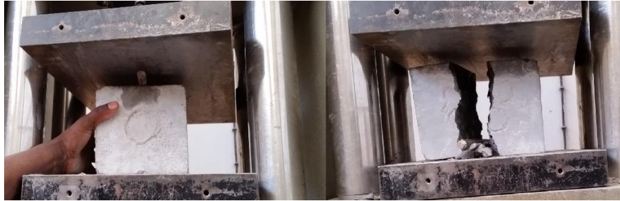
Figure 5.10. A concrete cube passing water penetration test when ready to be split (left) and after it was split (right).
