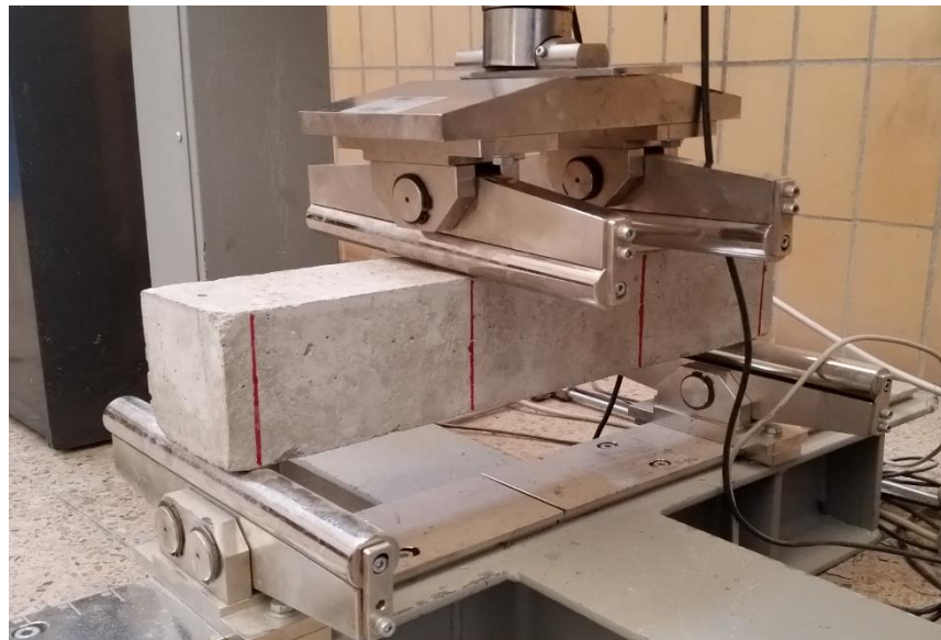
Figure 4.2. Concrete beam prepared for flexural strength test (Third point loading).
