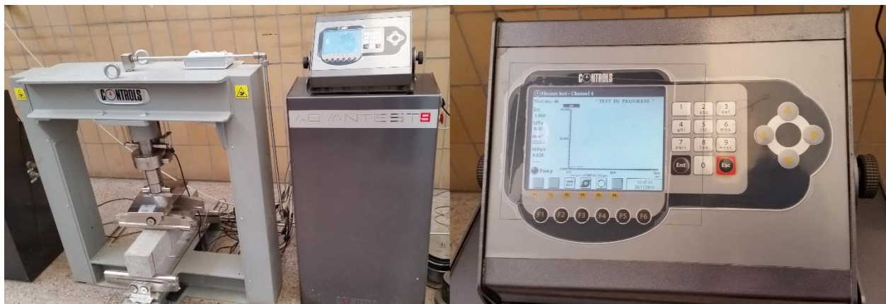
Figure 5.1. A concrete beam under flexural strength test (left) and data recorded in the display board (right)
