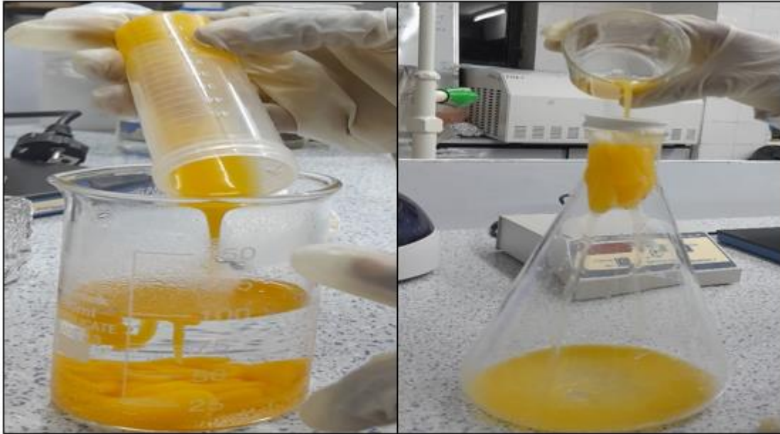
Mixing the egg yolk with pre-prepared media followed by filtration on clean flask
