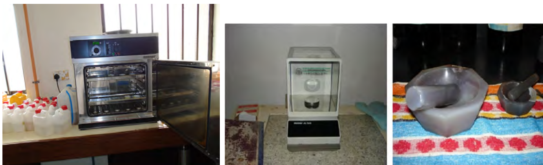
Figure 3.8: Standard oven with Figure 3.9: Four-digit Meter model weighing balance (on left side) and Agate Mortar (on right side)
