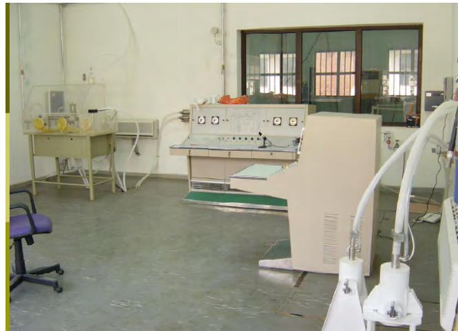
Figure 3.2: The Pneumatic Rabbit System for sample sending and retrieving out the reactor
