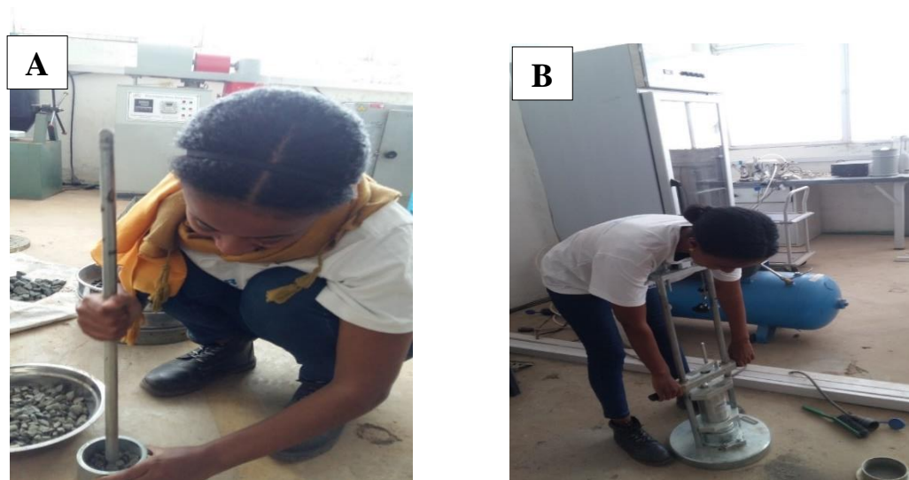
Fig 4.3: Sample Preparation for crushing value test (A) and Performing impact value test (B)
