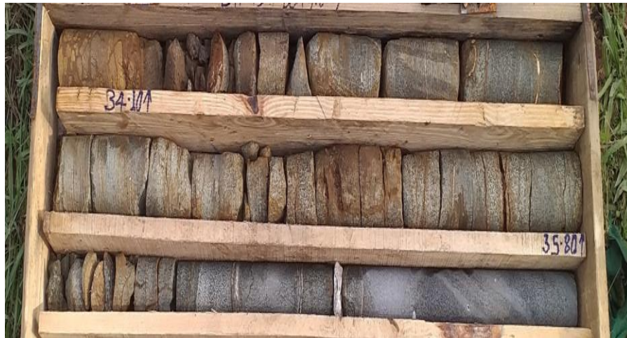
Fig 5.16: Core sample with poor RQD value
