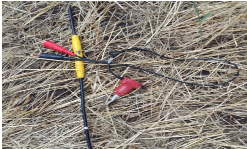
Fig 2.19: A single Geophone along with geophone cable
