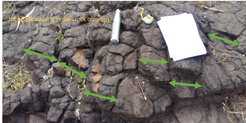
Fig 2.9: Joint Spacing of rock outcrop at a certain rock mass (Location: Project site, Proposed Intake section of the Tunnel Route)
