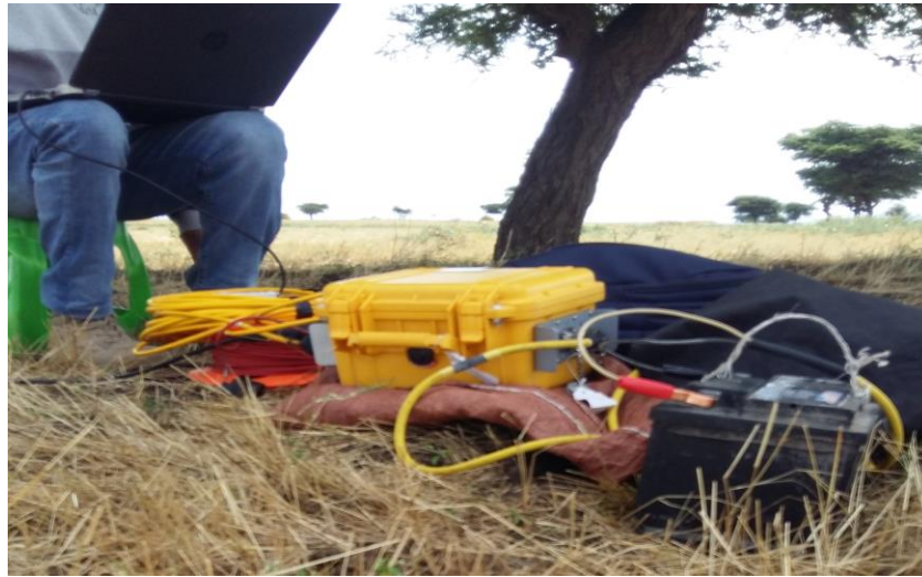
Fig 2.20: Seismograph (Seis-24) used to measure the compressional wave velocity
