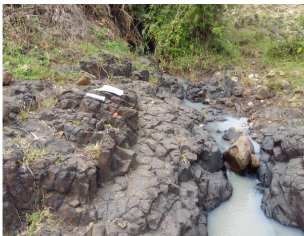
Fig 5.18: Very Blocky and Blocky Rock mass observed from field RMR points
