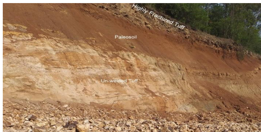
Fig 2.2: Stratified rock of varying structure, composition and grain size (Tuff) (Zone of unconformity) (Location: Proposed project site, Proposed Spillway Section)
