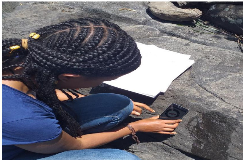
Fig 2.8: Measuring the orientation of a Joint face (Location: Project site, Proposed Inlet Section of the Tunnel Route)
