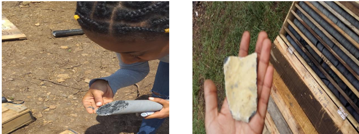
Fig 2.11: Calcite infillings obtained from drilled rock core sample (Location: Project site, BH-07)
