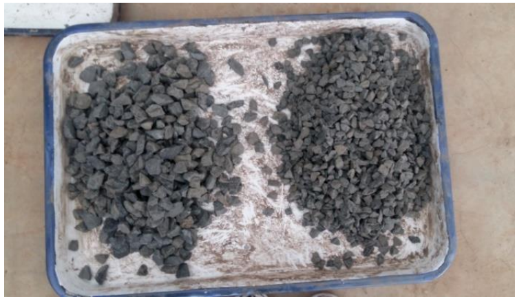
Fig 4.4: Prepared sample for LAA test
