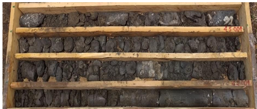
Fig 5.20: Zone of weakness in a rock core, highly decomposed and fractured at contact zones (BH-07, Dam section)
