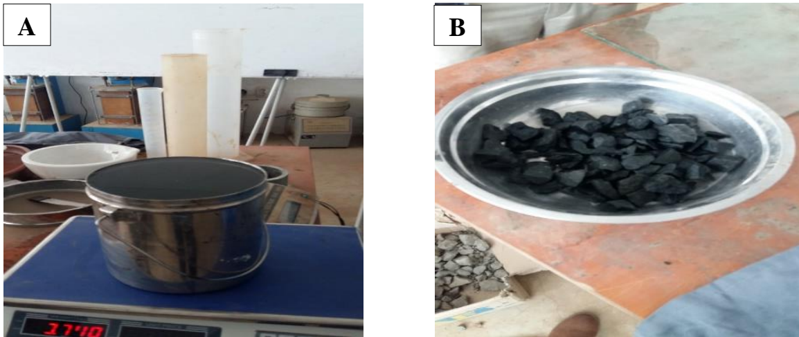
Fig 4.2: Soaked (A) and SSD (B) aggregate sample to determine Relative density and Water Absorption
