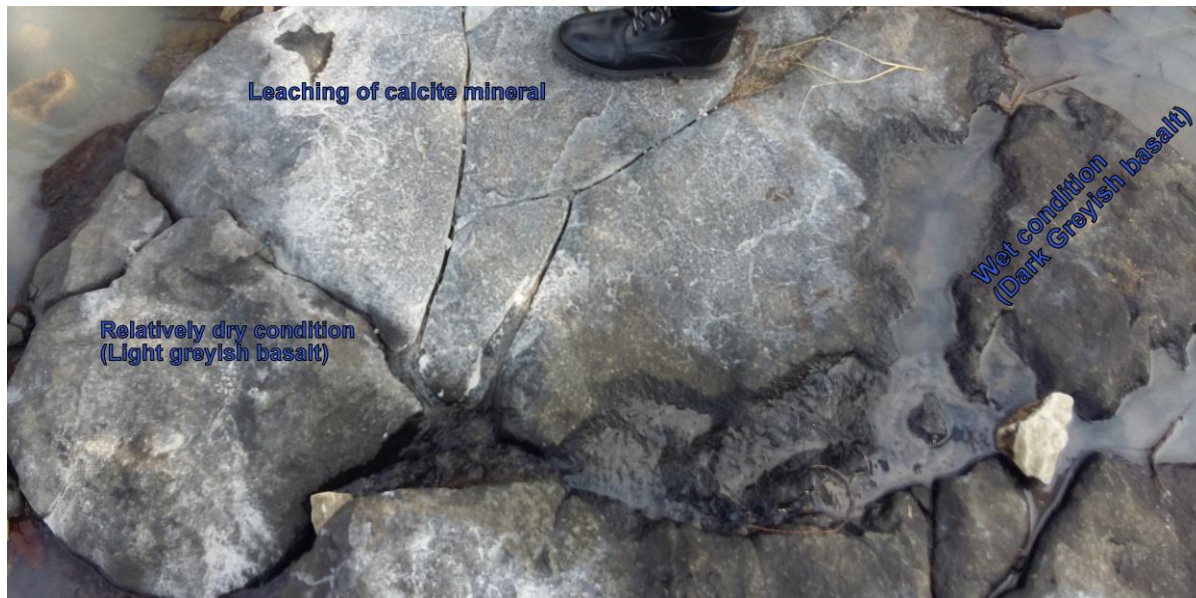
Fig 2.4: Variation in color of exposed rock unit under dry and weight condition (Location: Project site, Proposed Inlet Section of the Tunnel Route)
