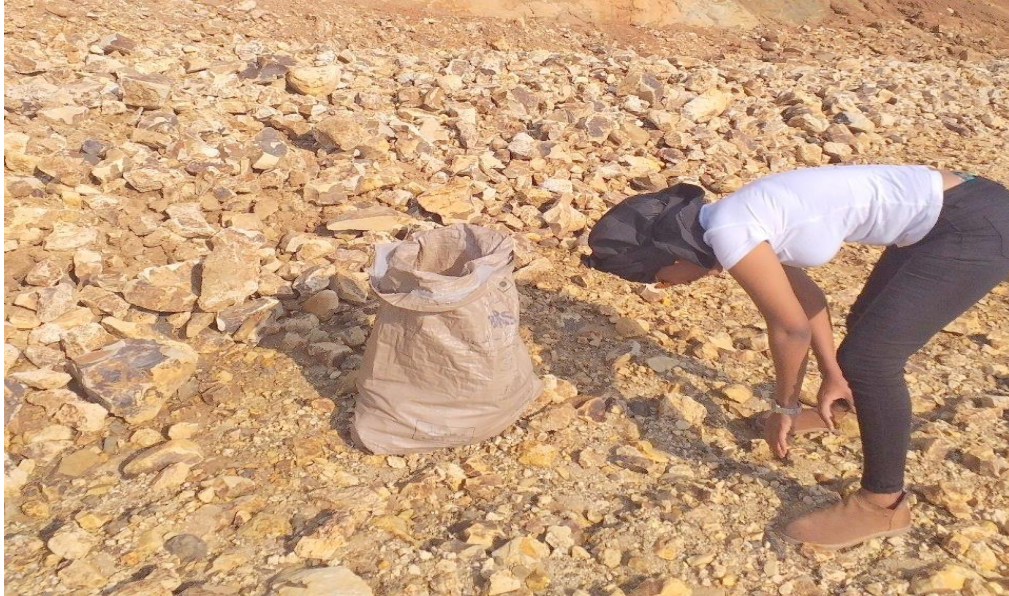
Fig 2.3: Relatively Hard and Strong Tuffaceous Rock material (Location: Project site, Proposed Spillway Section)
