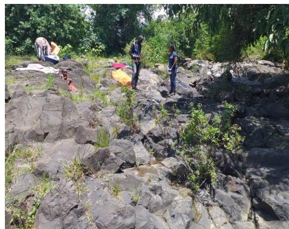
Fig 5.18: Very Blocky and Blocky Rock mass observed from field RMR points
