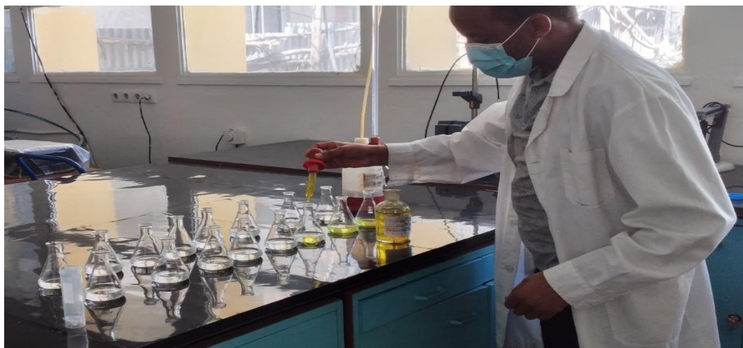
Figure 3: Experimental analysis of Argentometric titration method - Chloride
