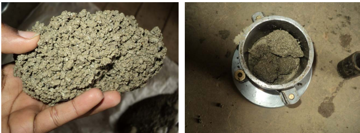
Figure 5.1.3.1(b) Agglomeration effect of sodium silicate
