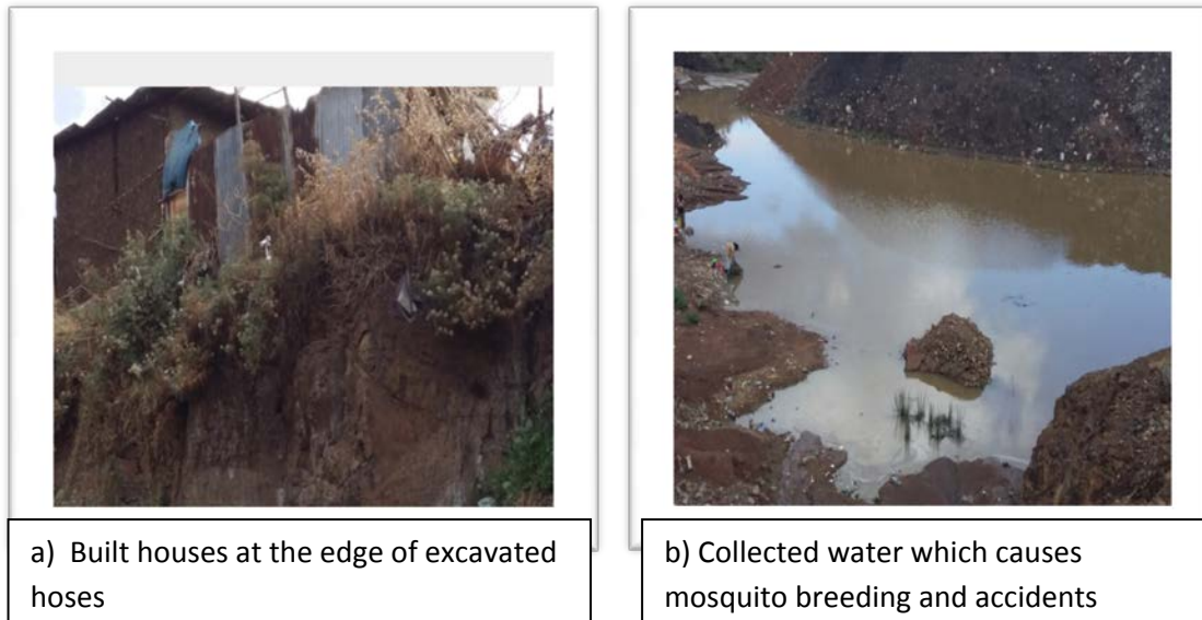
Figure 5 Risks of quarrying to the local community due to collected water and settlement at the edge of the pit
