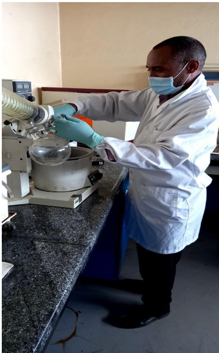
6. Adjusted Rota evaporator for concentration process.
