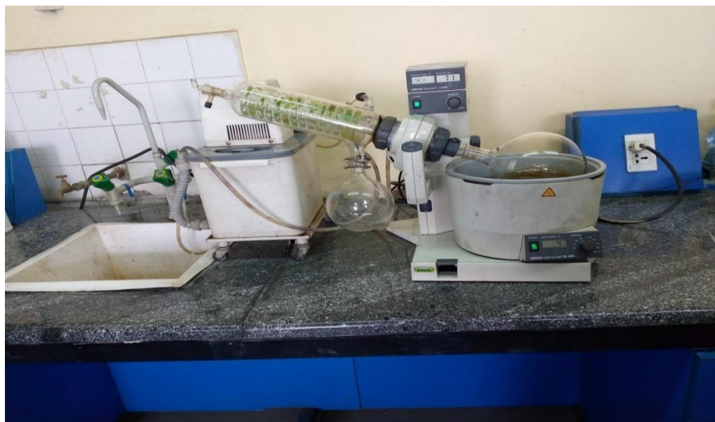
5. Buchi rota vapor (on condensation process)
