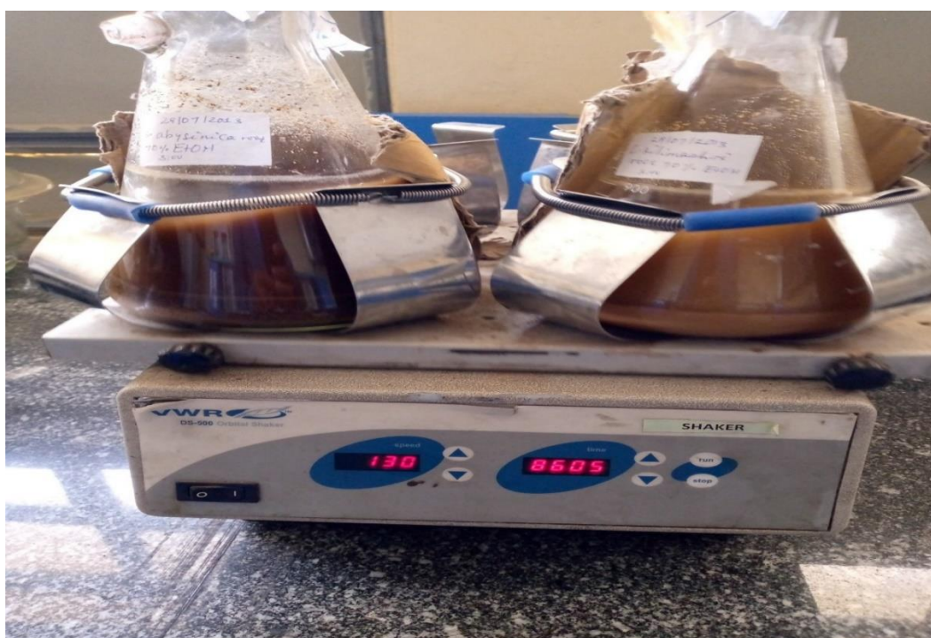
4. Rotary shaker adjusted at 130rpm
