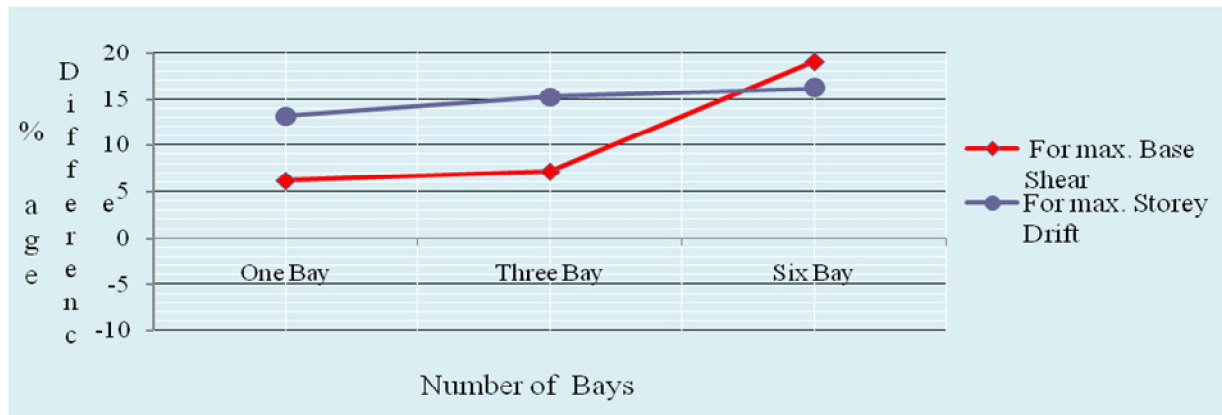
Figure 3-15 Percentage difference for base shear and drift of six storey frames
