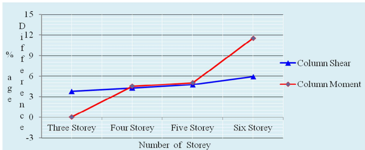
Figure 3-12 Percentage difference for column member moment of three bay frame
