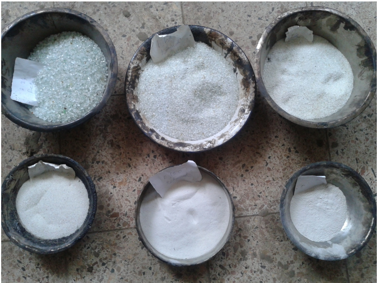
Crushed glass with different sieve size
