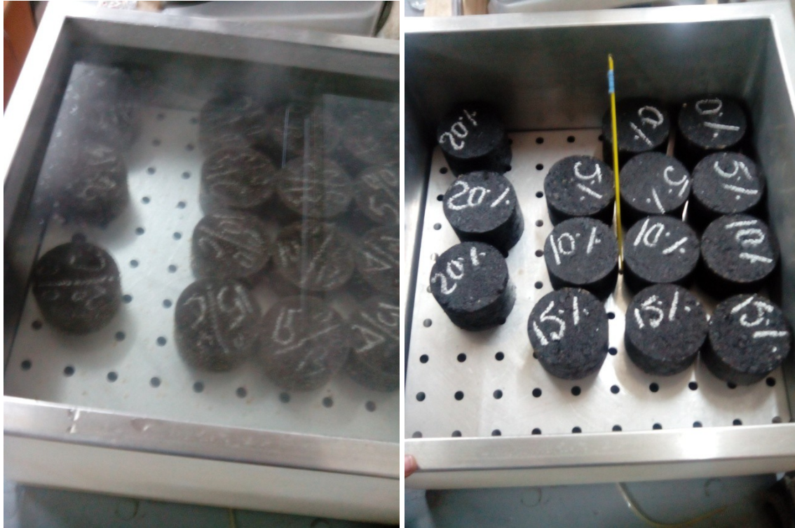
Samples in water and air bath for Marshall Immersion Test
