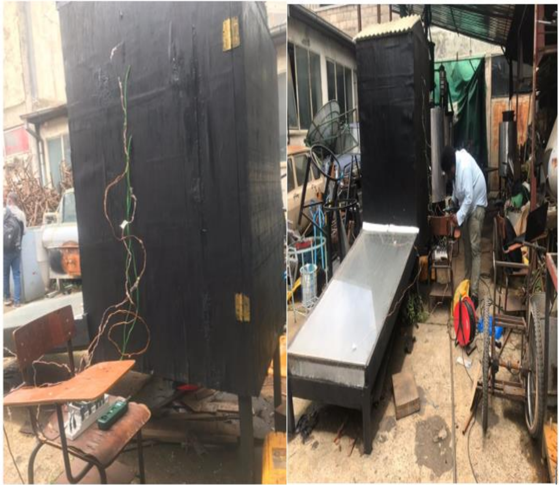
Figure 6.15: Instrument Setup for the Modified Mixed Mode Drier
