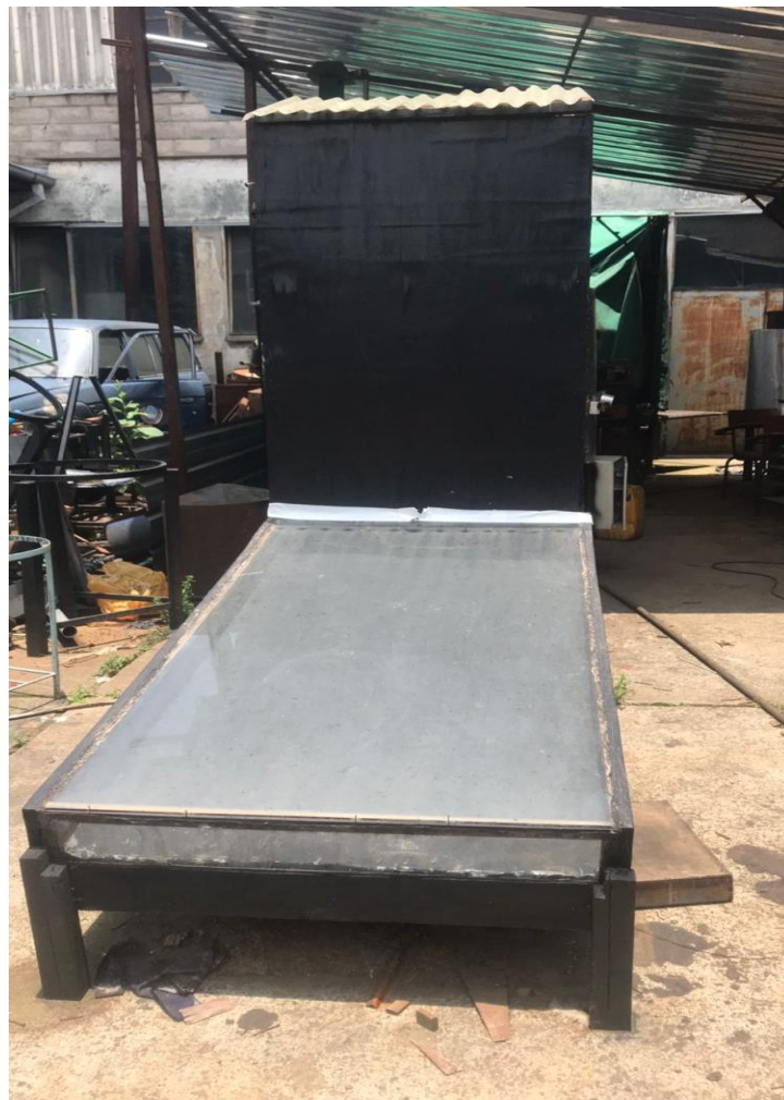
Figure 3.1: The Prototype Solar Injera Drier
