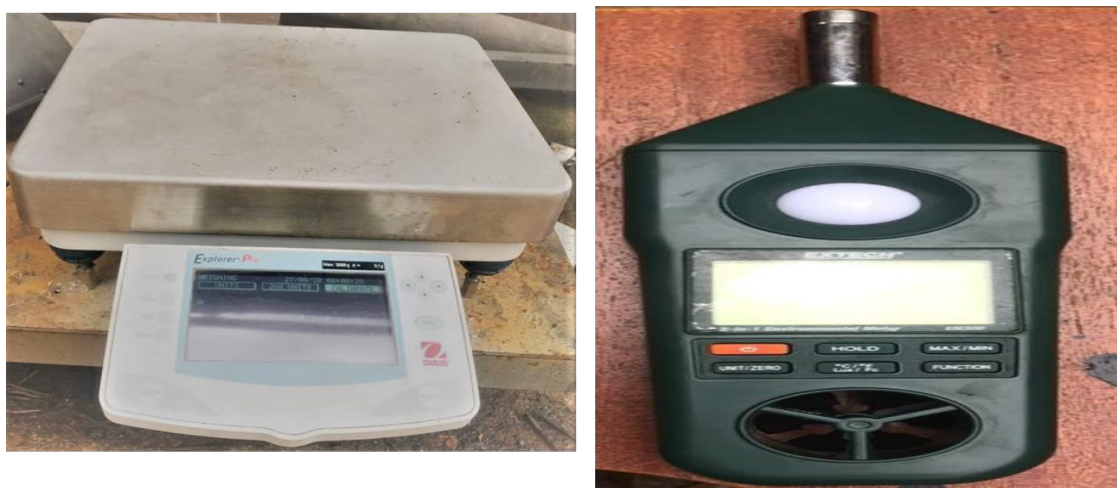
Figure 5.3:Weighing Balance and Velocity and Temperature Measuring Device
