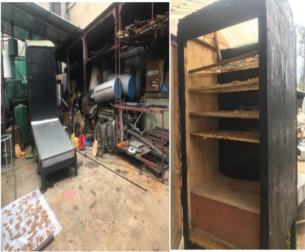
Figure 6.13: Experimental Setup for the Modified Mixed Mode Drier
