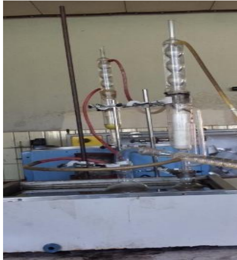
Figure 3.1: soxhlet extraction unit set up
