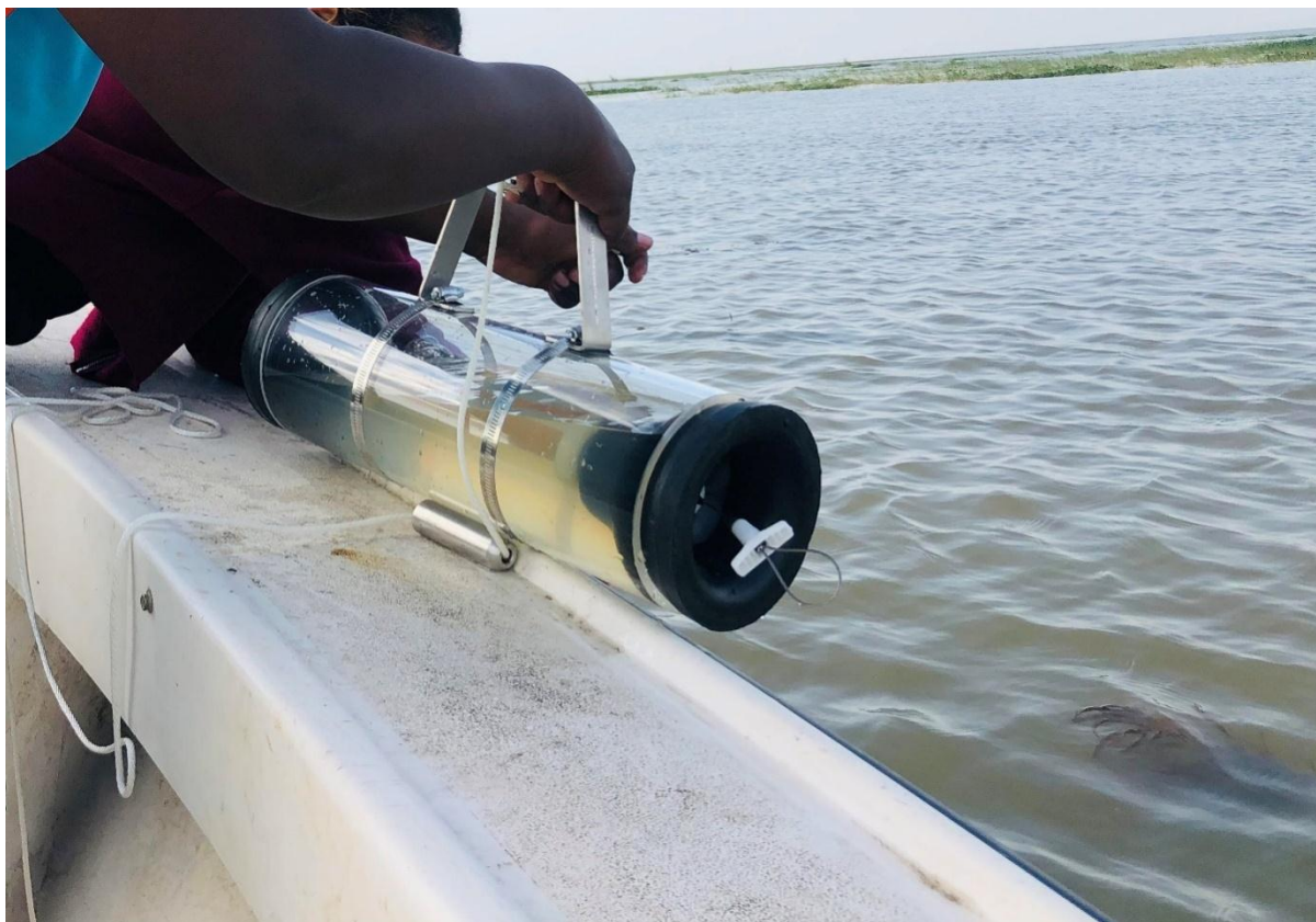
Figure 13: Collection of water samples using a bottom water sampler
