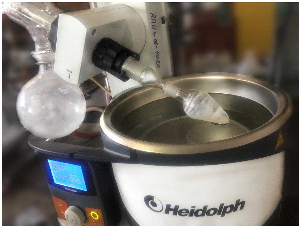
Figure 16: Concentration of samples extract in a rotary evaporator
