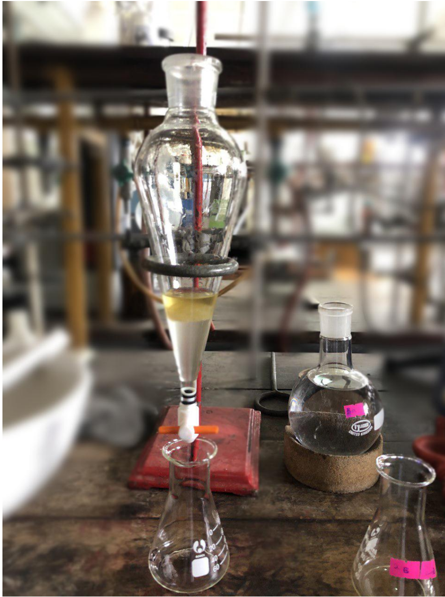
Figure 15: Liquid-Liquid extraction of the 2,4-D acid
