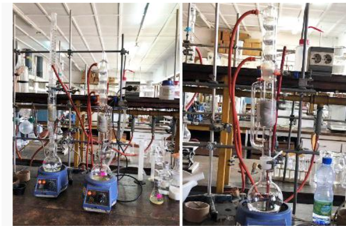
Figure 17: Soxhlet extraction of soil samples
