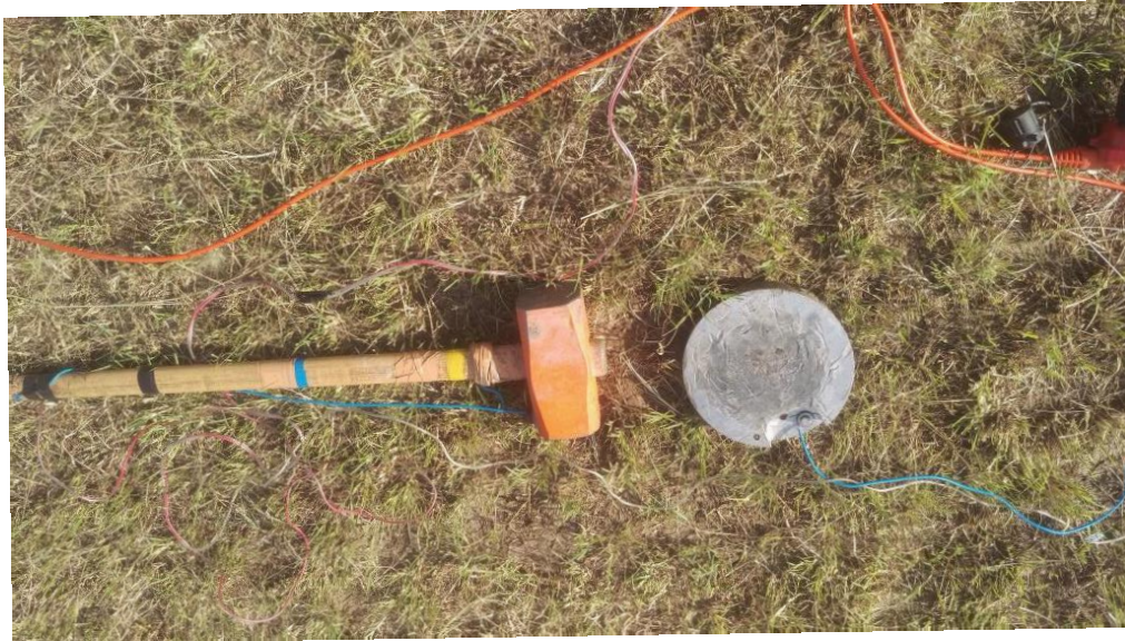
Figure 5.5 sledgehammer and metal plate used for seismic refraction survey
