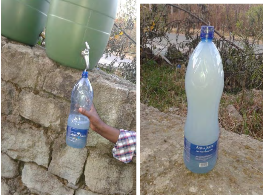
After a 2-day detention time take treated grey water for laboratory test
