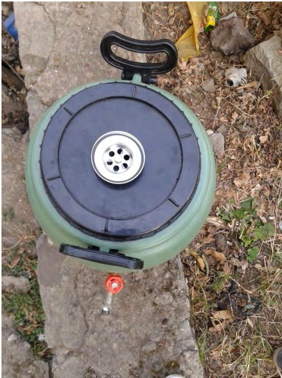
The first barrel is ready to store untreated grey water collect untreated grey water from cloth washing
