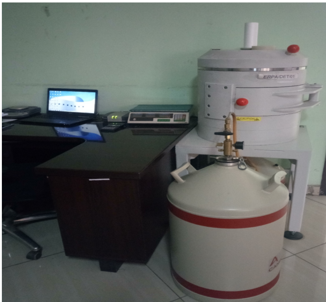
Figure 3.3. Gamma spectrometry mounted with HPGe detector and DSA circuit (ERPA Lab.)
