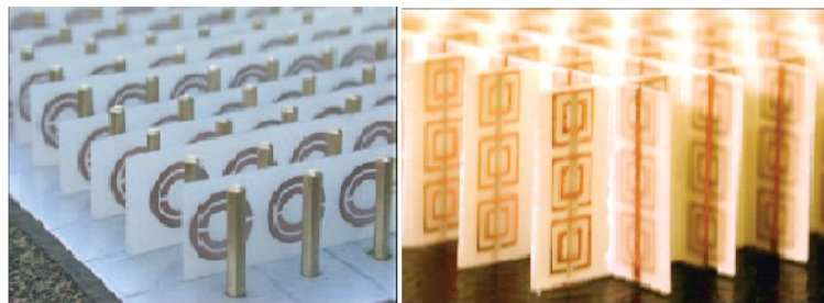
Figure 2.5: SRR-thin array of long metallic wires.
