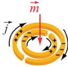
Figure 2.8: When a magnetic field parallel to the ring axis is switched on it induces currents in the “split rings”.
