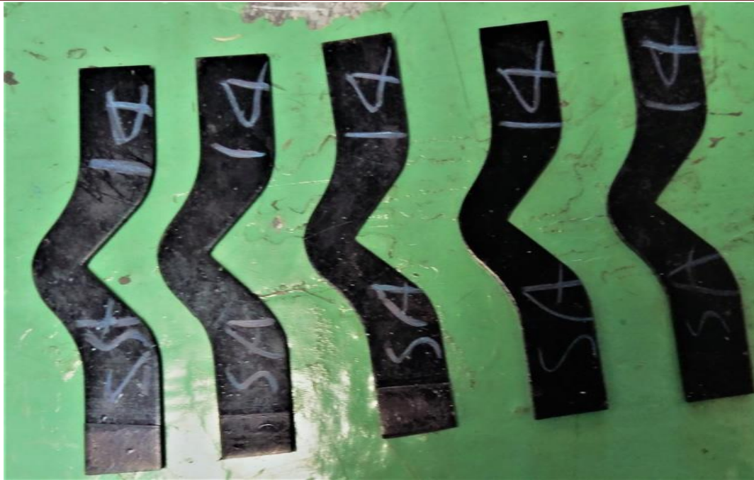
Figure 3.3.8 b. Sample Rubber membrane for Tear or Cohesion Test at Horizon Laboratory
