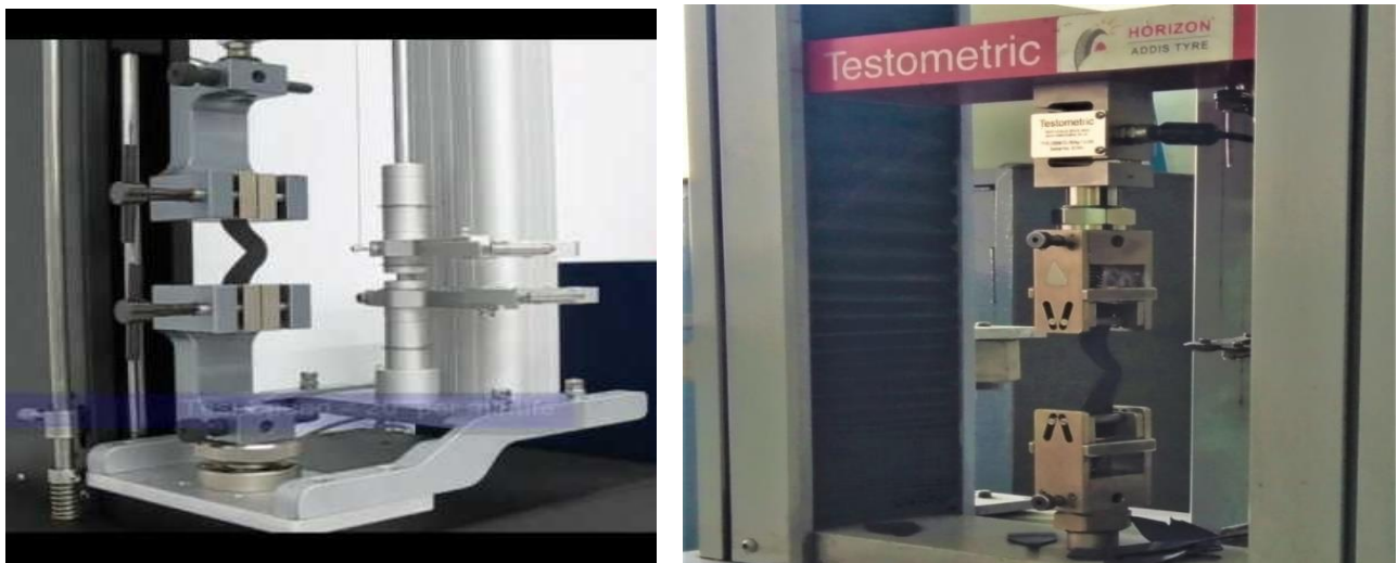
Figures 3.2.8 cohesion or tear strength testing equipment
