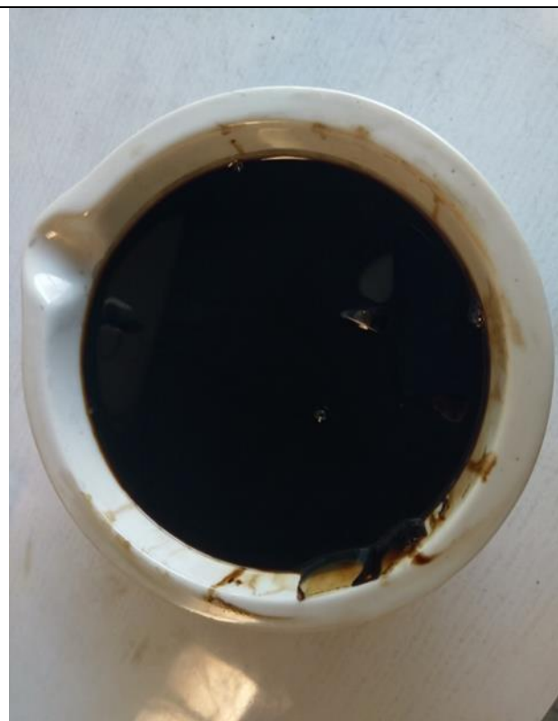
Figure 50. Specimen has been dissolved after oil immersion test
