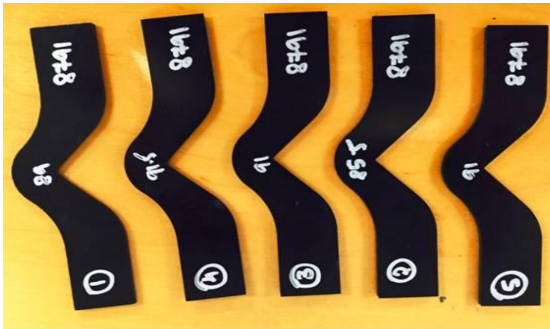
Figure 3.3.8 a. Sample of Rubber membrane for Tear or Cohesion Test (ASTM D624)
