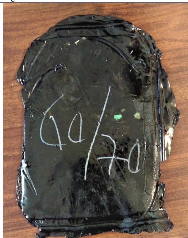
Figure 40. Specimen of Sand and Bitumen after curing
