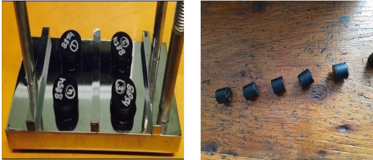
Figure 3.3.2 Sample preparation for Compression Set as per ASTM and Horizon Lab
