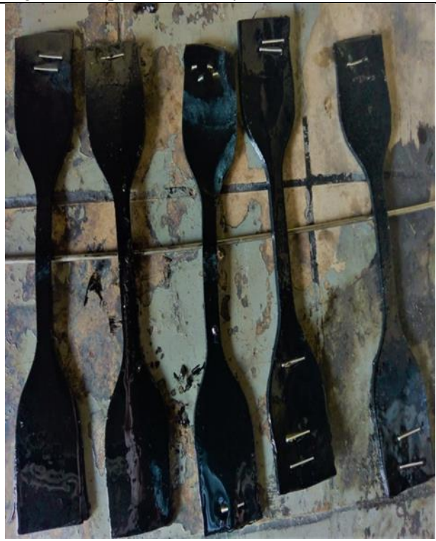
Figure 36. Specimen after oil immersion test
