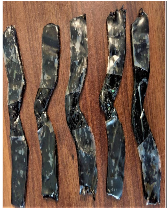
Figure 42. Type C or Right angle Tear Specimen for Mixture of Sand and Bitumen
