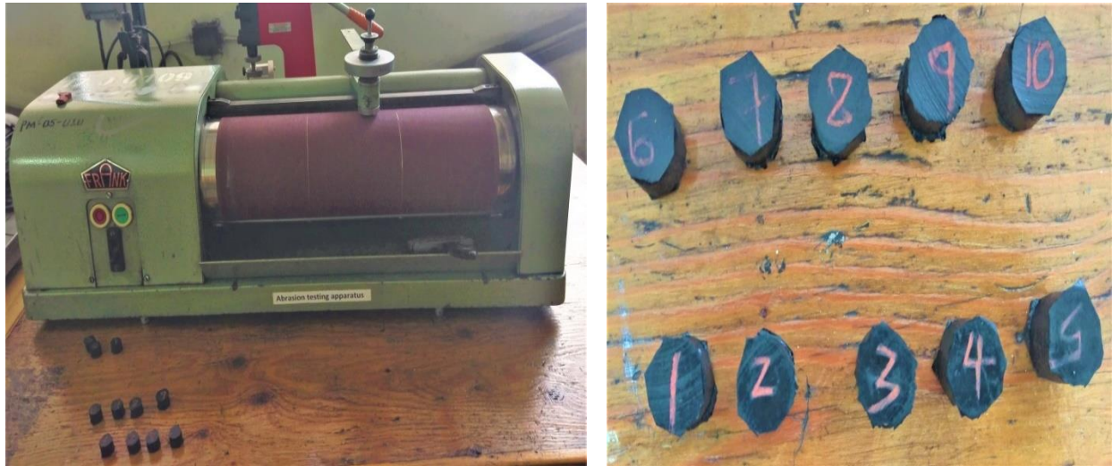
Figure 3.3.4 Sample and test equipment set up for Abrasion
