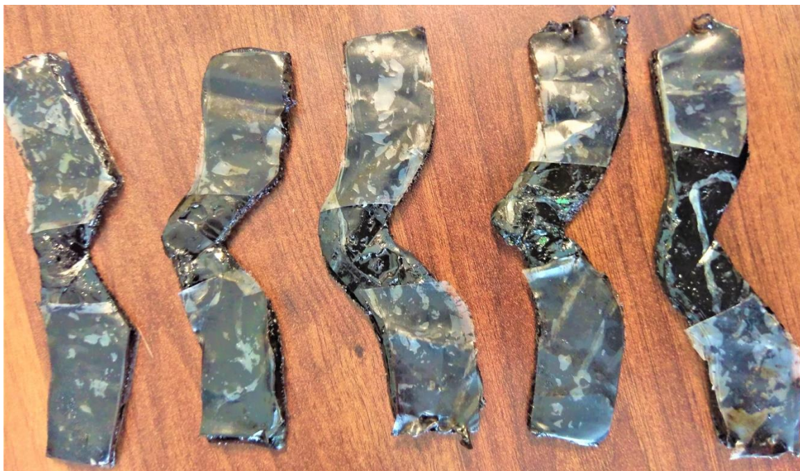
Figure 3.3.8 c. Sample bitumen-san mix for Tear or Cohesion Test at Horizon Laboratory
