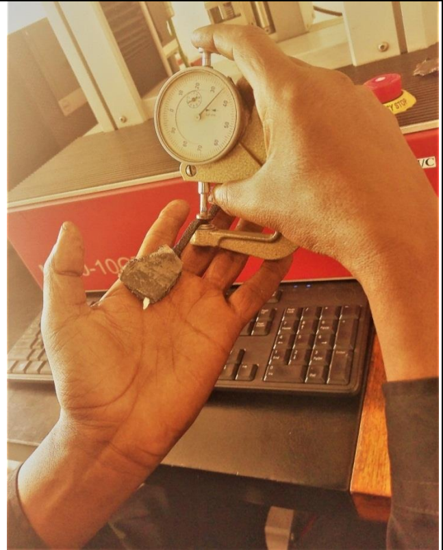
Figure 44. Specimen thickness measurement
