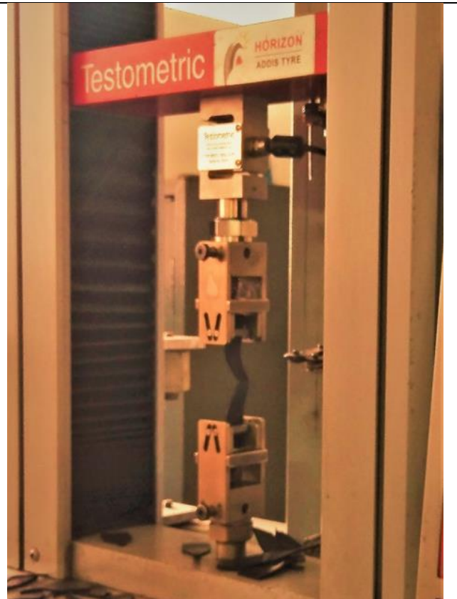
Figure 22. Tear (Cohesion) test on progress
