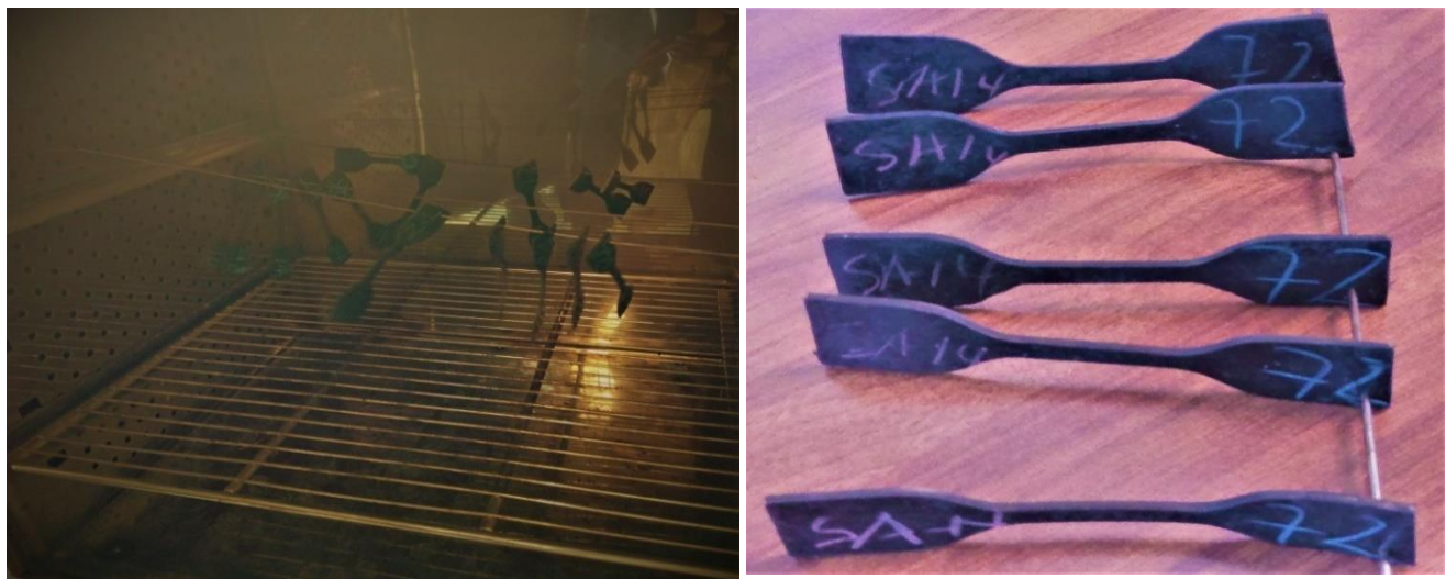
Figure 3.3.4 Sample Set up inside and outside oven for heat resistance
