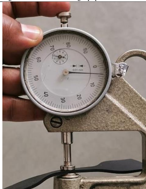
Figure 20. Specimen thickness measurement for Rubber membrane
