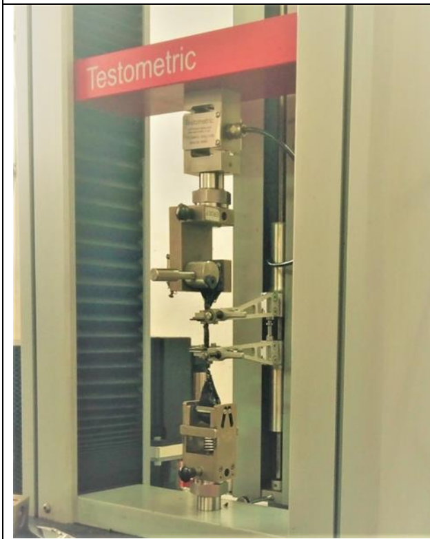
Figure 47. Elongation test on progress for Mixture of Sand and Bitumen
