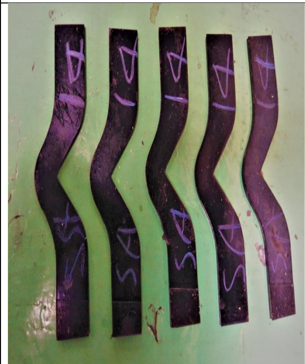
Figure 15. Type C or Right angle Tear Specimen for rubber membrane
