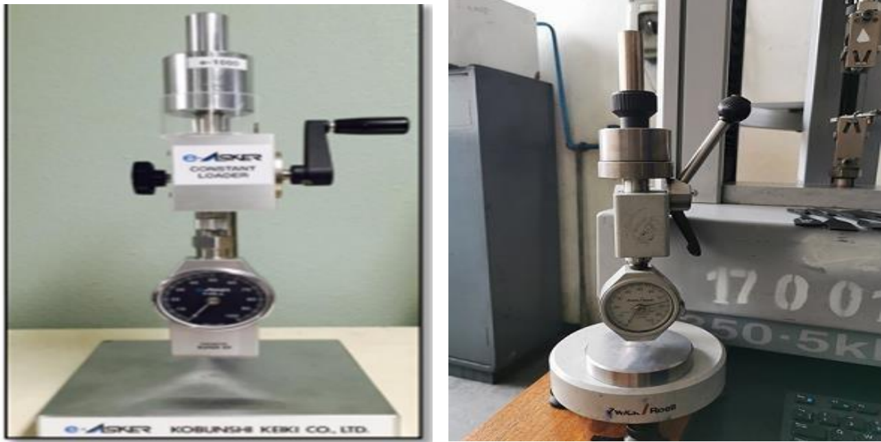
Figure 3.2.1 Hardness testing equipment (ASTM) and Horizon Addis Tire Lab respectively
