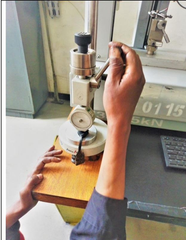
Figure 43. Specimen Hardness Measurement for Mixture of Sand and Bitumen
