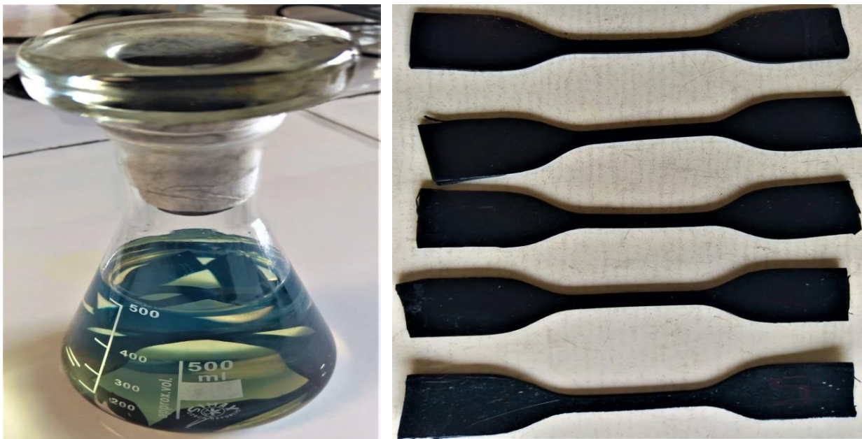
Figure 3.3.6 Sample Set up inside and outside diesel fuel for Oil resistance
