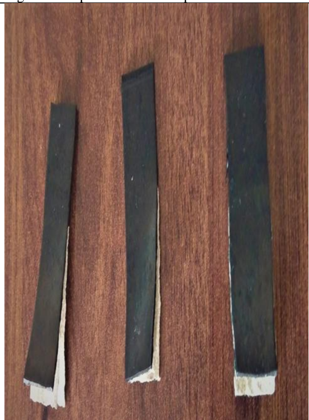
Figure 28. Specimen for Adhesion Test
