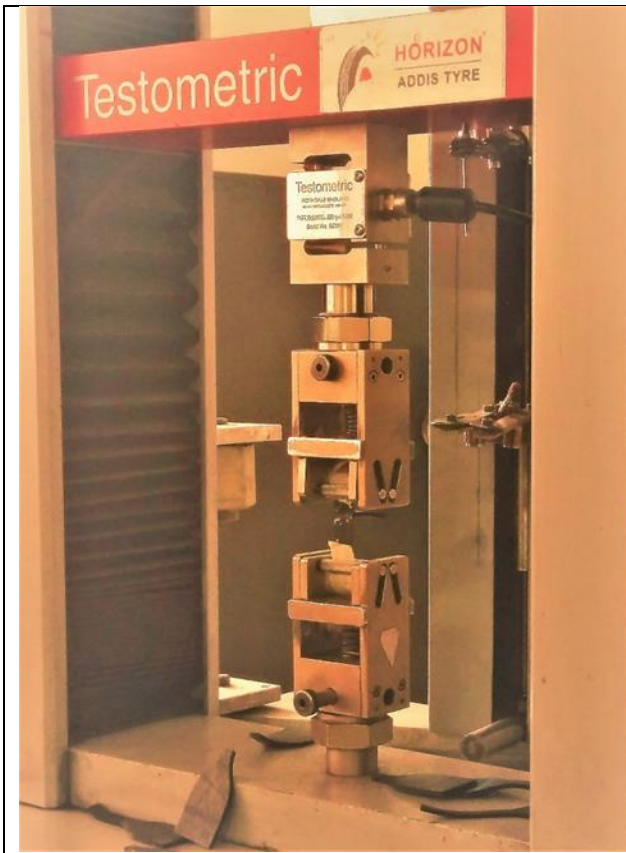
Figure 29. Adhesion test on progress
