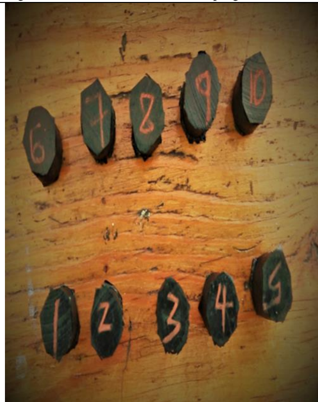
Figure 24. Specimen for Abrasion Test
