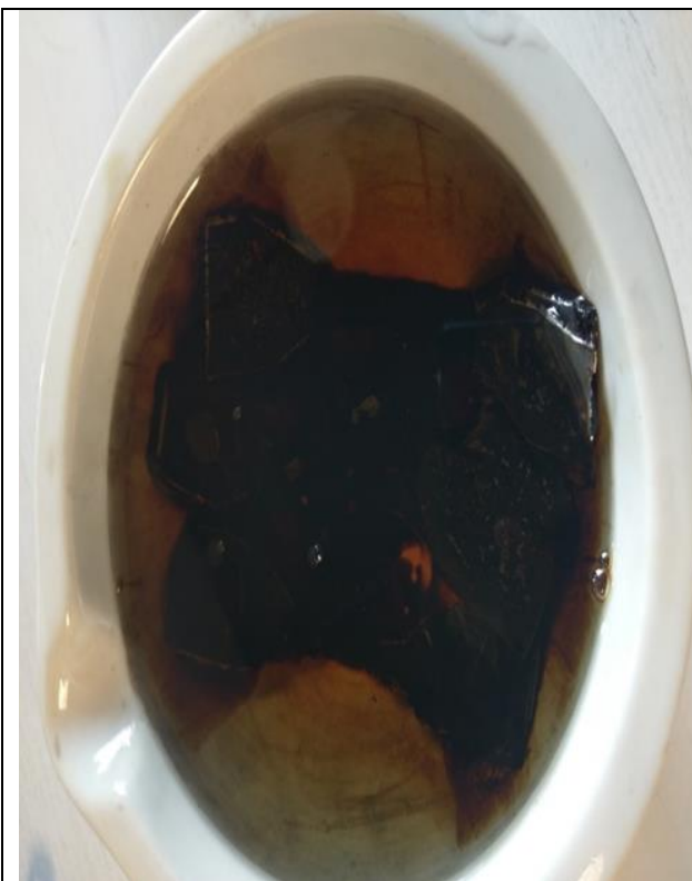
Figure 49. Specimen immersed in ASTM Reference Fuel (F), Diesel fuel
