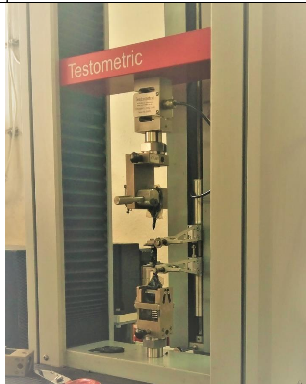
Figure 48. Elongation test sample @ break point
