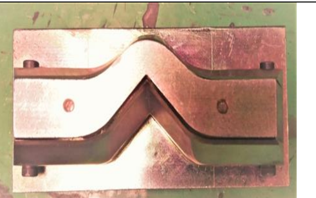
Figure 12. Cutting mold for dumbbell and tear, Type-C specimen respectively
