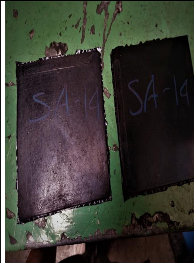
Figure 13. The specimens after curing
