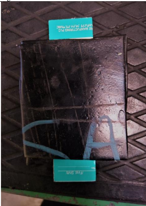
Figure 27 . Specimen before curing for Adhesion Test
