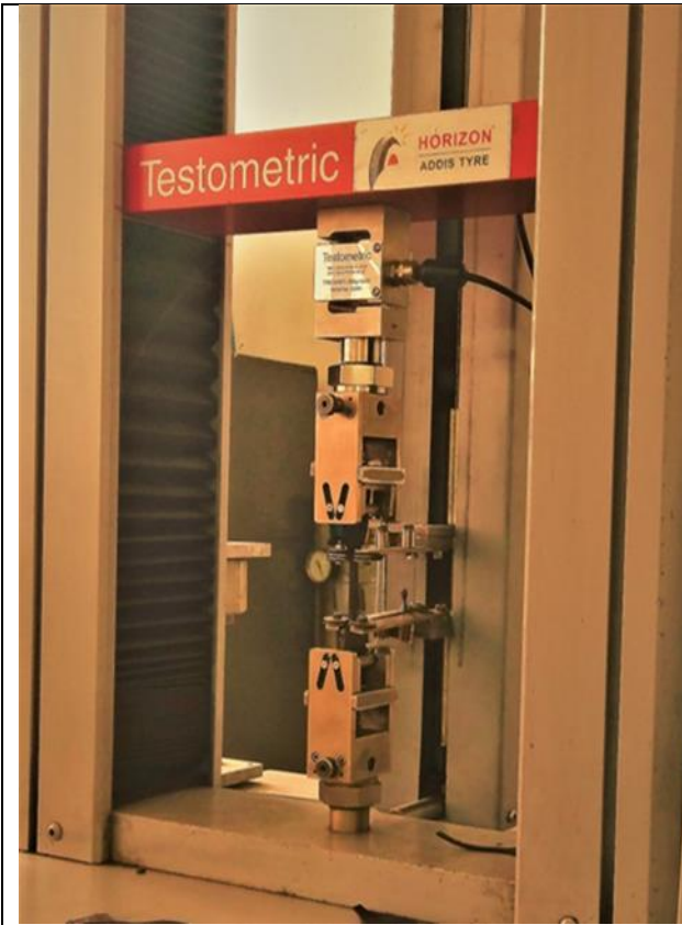
Figure 21. Elongation test on progress
