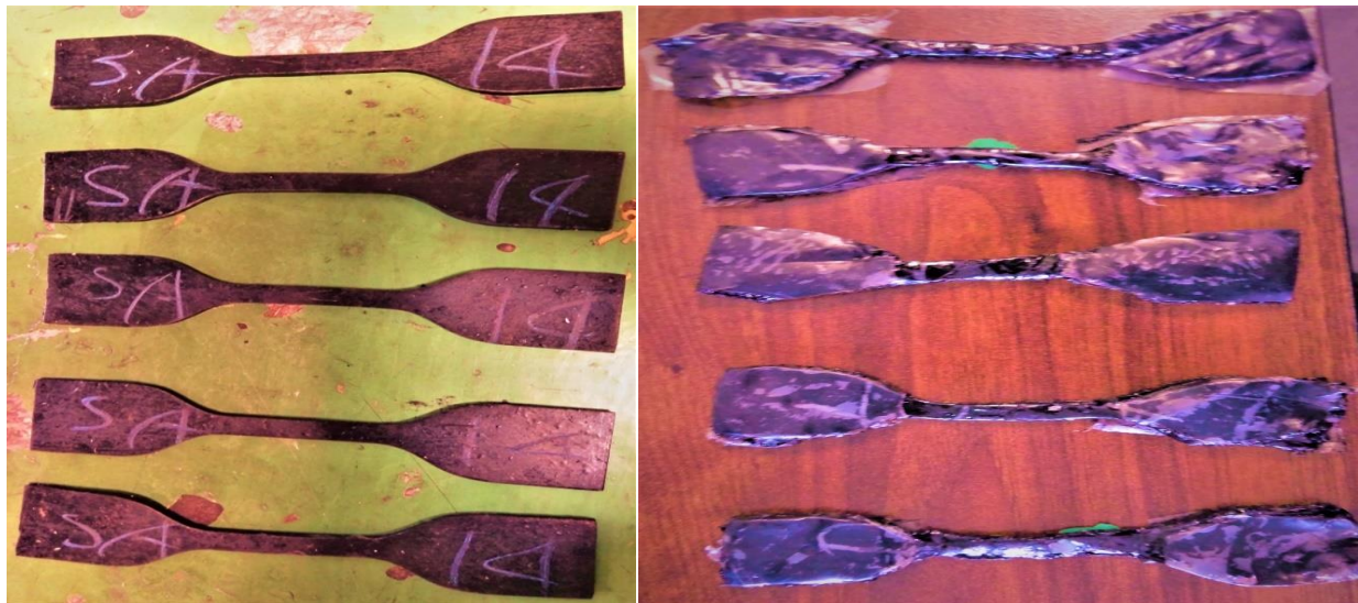
Figure 3.3.1 Dumbbell specimens of rubber membrane and sand-bitumen mix
