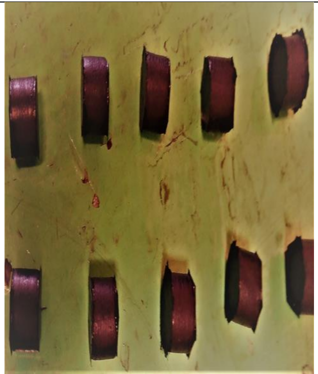
Figure 26. Specimen for Compression Test
