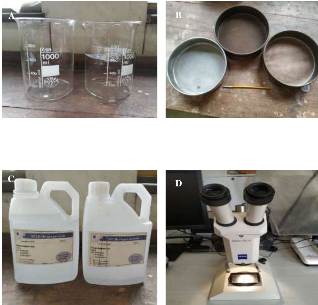
Figure 3.1 photographs show the laboratory instruments A) beaker B) sieves and brush C) H 2 O 2 D) Binocular microscope
