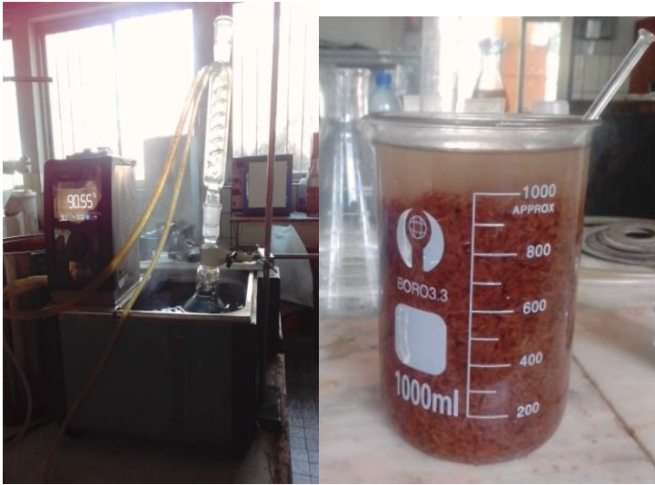
C1: Reflux condenser for acid treatment of RH
