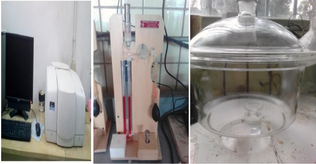
C10: FT-IR instrument C11: Air permeability blaine meter C12: Moisture absorptive test
