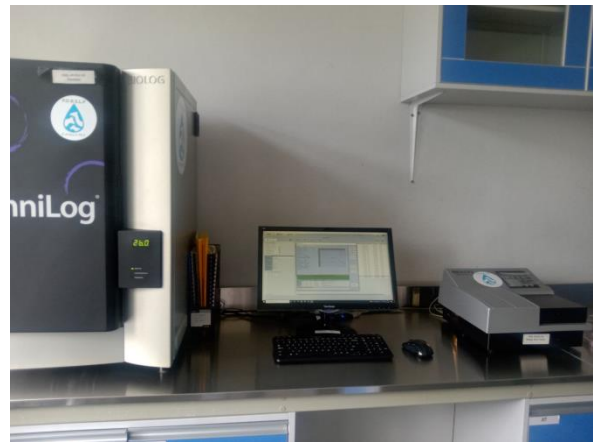
l) OmniLog for bacterial identification
