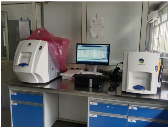
k) TEMPO ® machine for bacterial count
