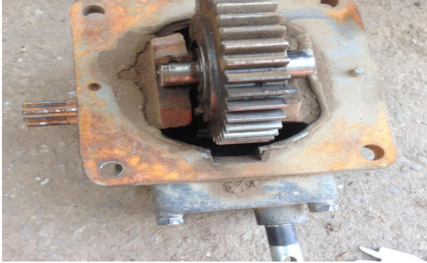
Figure 3.3 Chery 100hp failed transfer case
