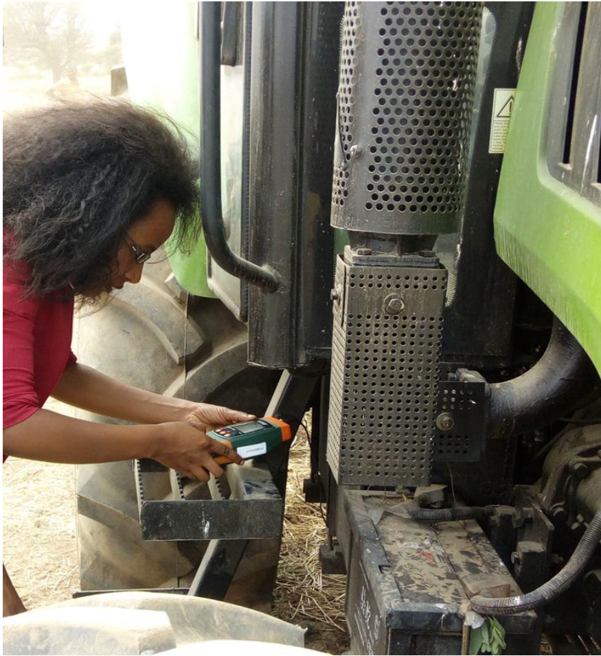
Figure 3.5 the vibration meter magnet tip attachment to transfer case
