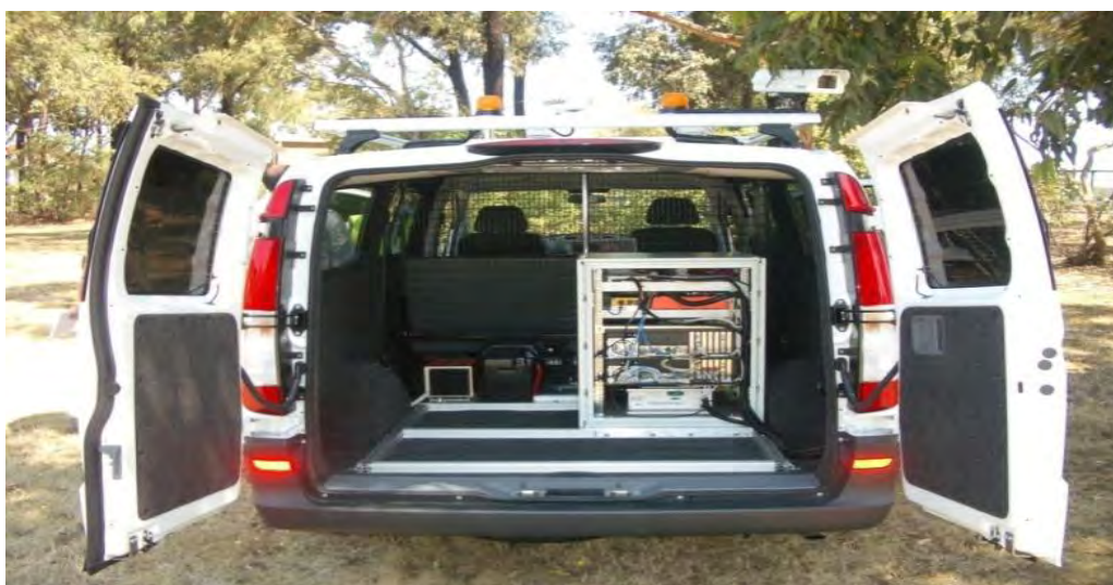
Figure 4.5: Hawkeye 2000 Road data collection equipment
