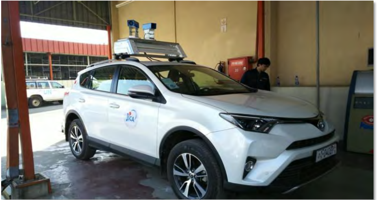
Figure 4.12(a): Pavement condition survey vehicle in AACRA
