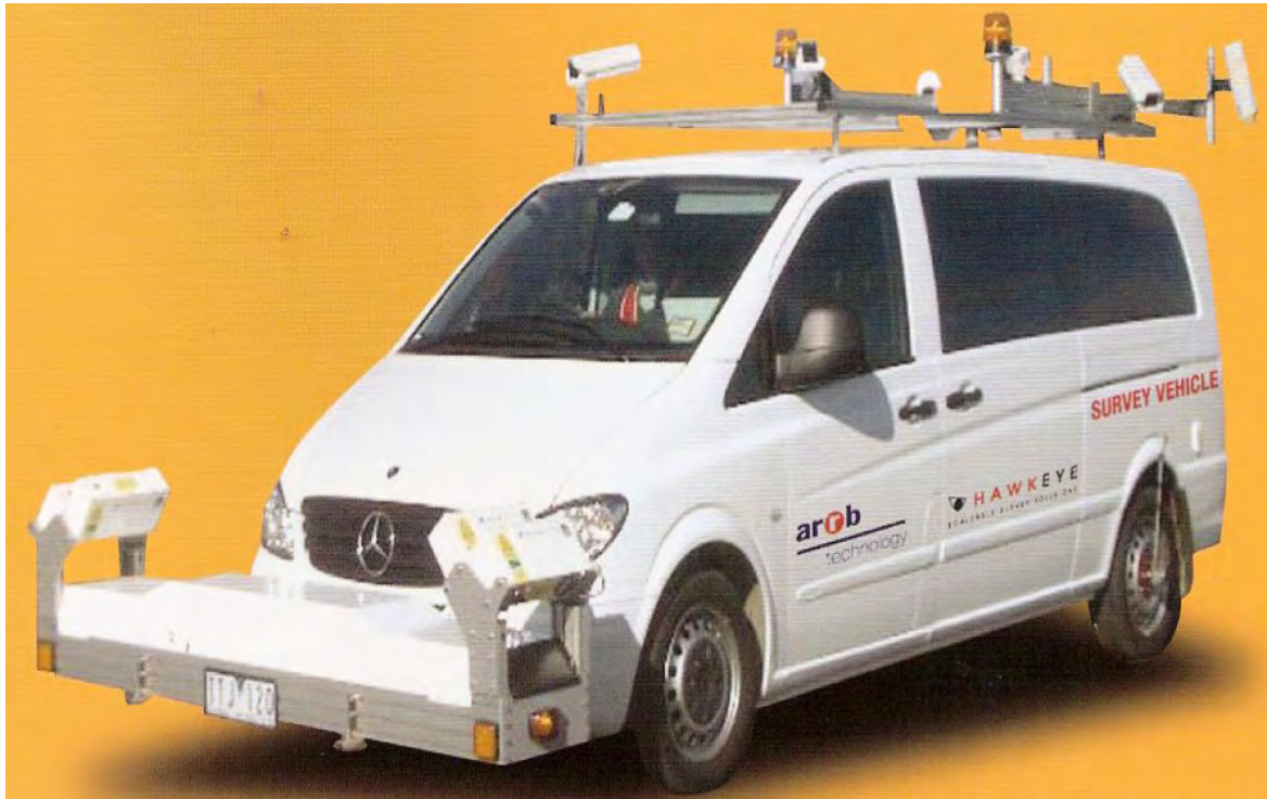
Figure 4.4: Hawkeye 2000 Road data collection equipment
