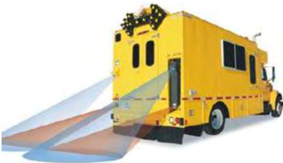
Figure 2.3: ARAN profile measurement systems
