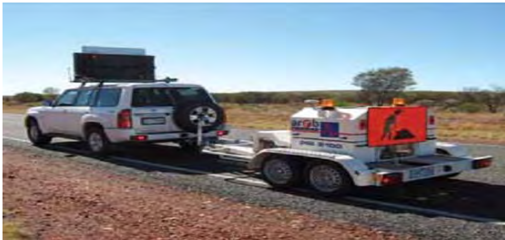
Figure 4.6: Falling Weight Deflectometer(FWD)
