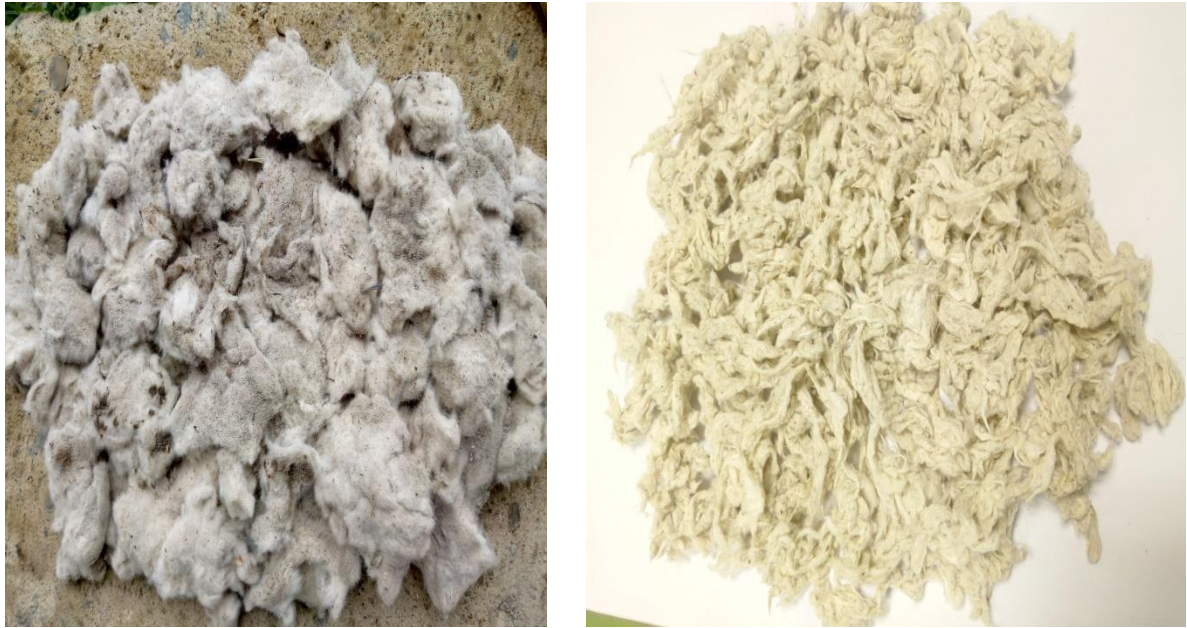
Figure 2: Images of Cotton linter uncleaned (left) and cleaned (right) taken from Dukam ginning factory (Photo by M. Teshome).
