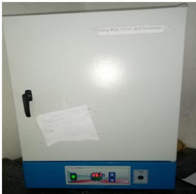
Drying the filtered cake in Oven and incubator at 105°C
