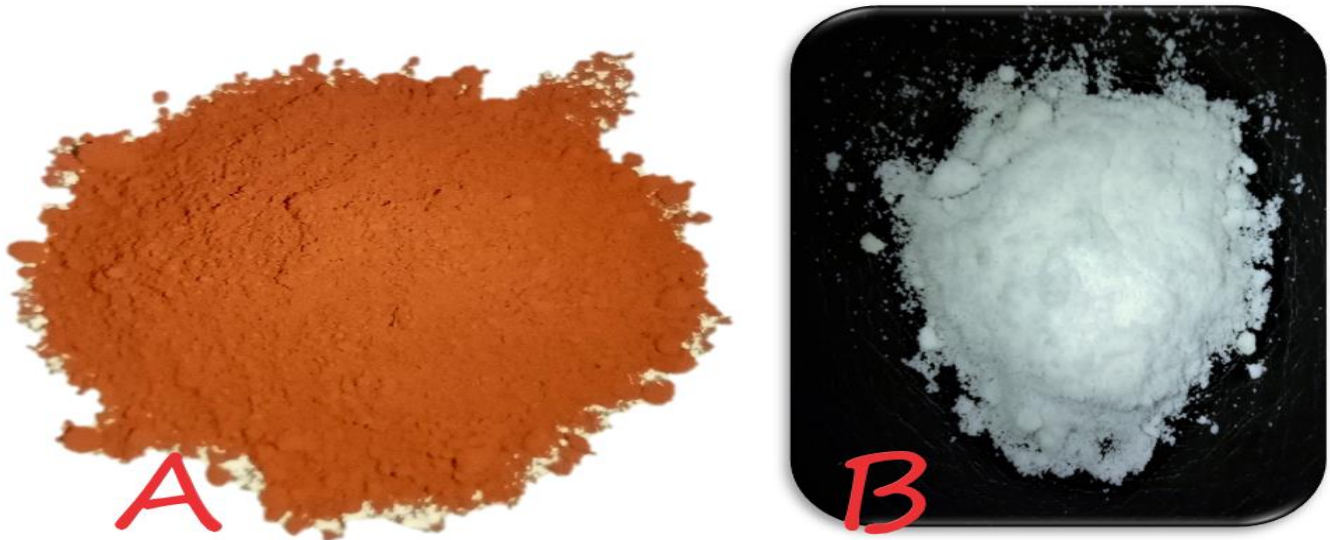
Figure 3.3: A) \alpha -ferric oxide (Product) and B) Ammonium chloride (Byproduct)
