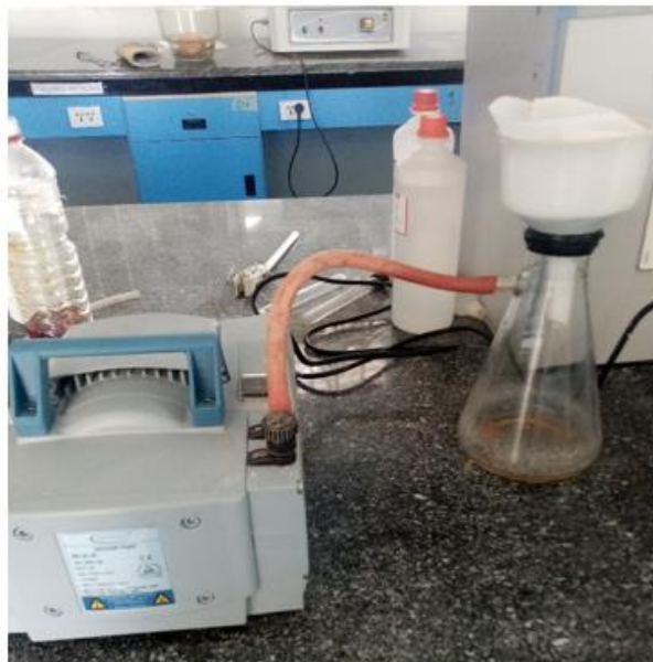
Filtering the cake formed in Vacuum pump
