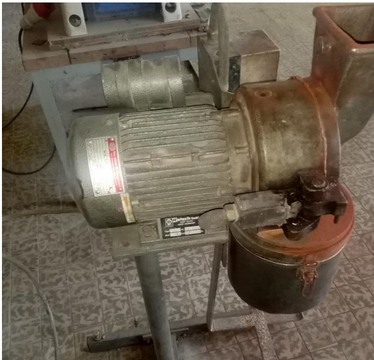
Milling the iron ore by RETSCH (5657 HAAN) miller
