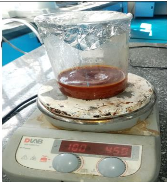
Reacting the ore with HCl in heater with magnetic stirrer
