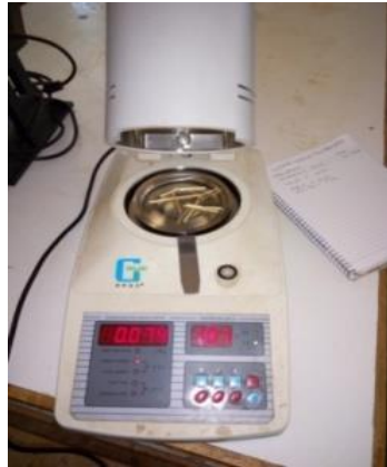
Figure 3. 2. Infrared Moisture Genis Photometer (Direct Moisture Tester)
