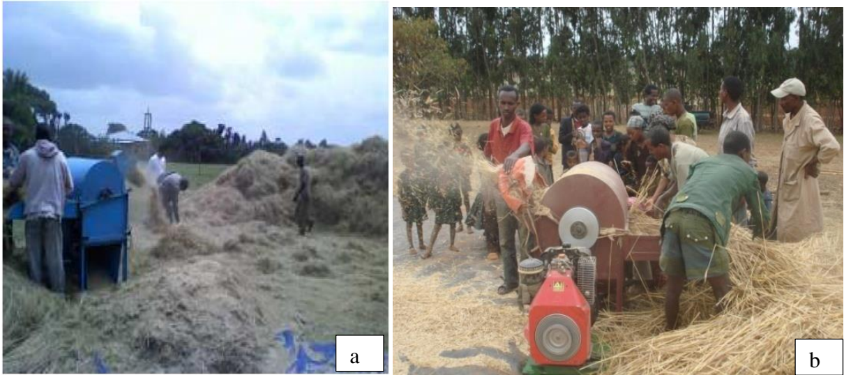
Figure 2. 6. Stationary threshers a) Bahirdar modified SG-2000 b) multi-crop thresher (through put type) in Ethiopia
