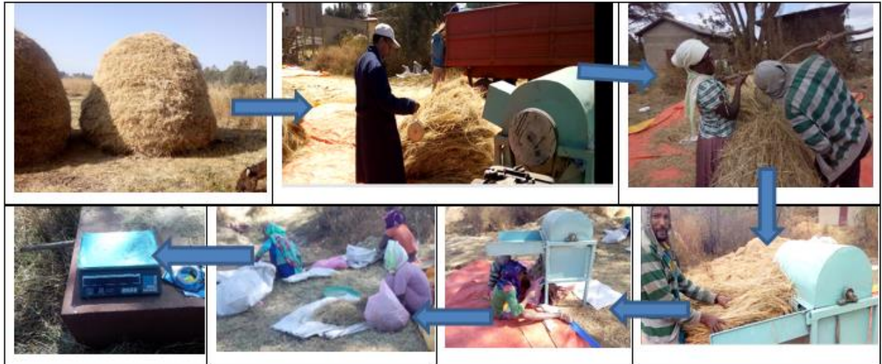
Figure 3. 9. Test procedures (from unthreshed sample preparation up to manual cleaning and separation of threshed samples (straw, chaff and tef mixture) from each sample box)
