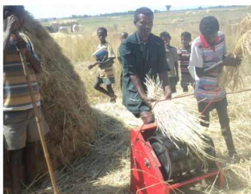
Figure 2.4. Human (labour) operated mechanical threshing system or hold-on rice thresher in Ethiopia
