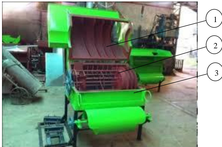
Figure 2. 7. Internal parts of stationary threshers SG-2000: 1.Drum cover 2. Drum (beater) 3. Concave
