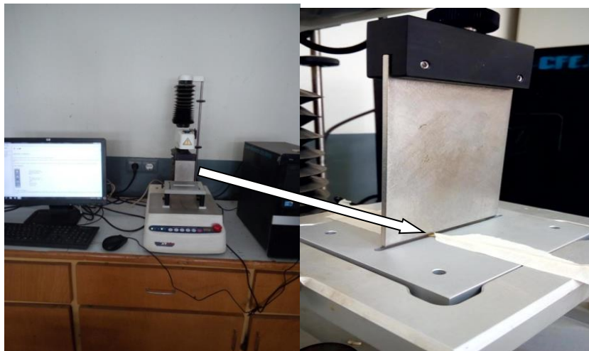
Figure 3. 5. Texture Analyzer TA.XTPlus with full computer accessories
