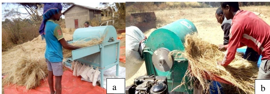
Figure 3. 10. Comparison of threshing units a) newly developed b) SG-2000 threshing unit
