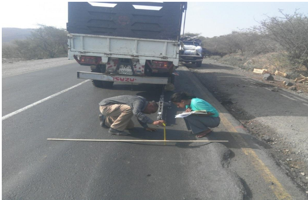
Figure 27. Rut Depth Measurement during Pavement Condition Survey
