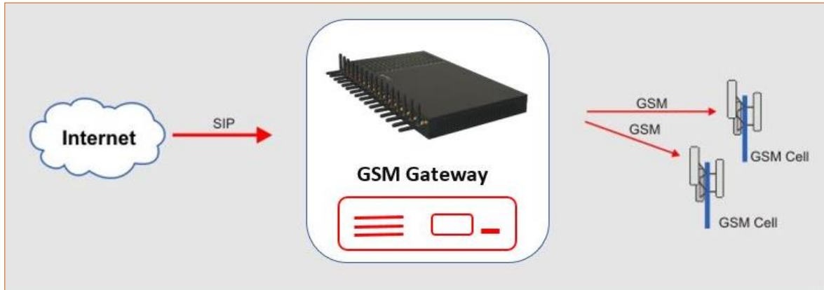
Figure 2.2: GSM gateway Termination Route
