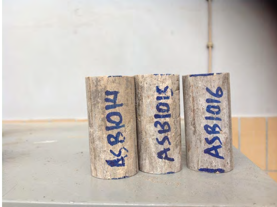
Figure 5-2: Sample Prepared for Compression
