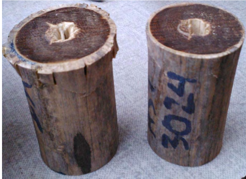
Figure 6-1: End bearing and Splitting Failure
