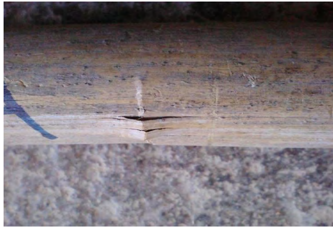
Figure 6-3 (a): Local cracking failure of Assosa bamboo
