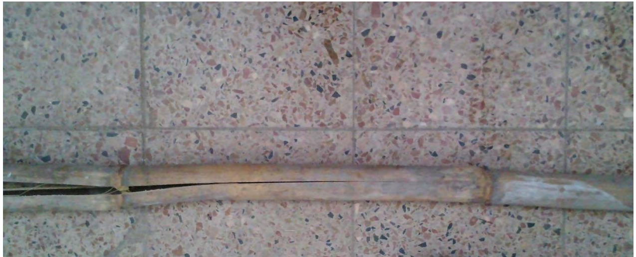
Figure 6-3(b): Splitting failure of Assosa Bamboo
