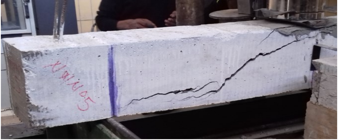
Figure 6:3: Diagonal tension failure in Specimen NWNo.5
