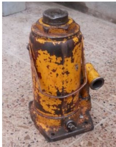
Figure 4:7: Load applying hydraulic jack
