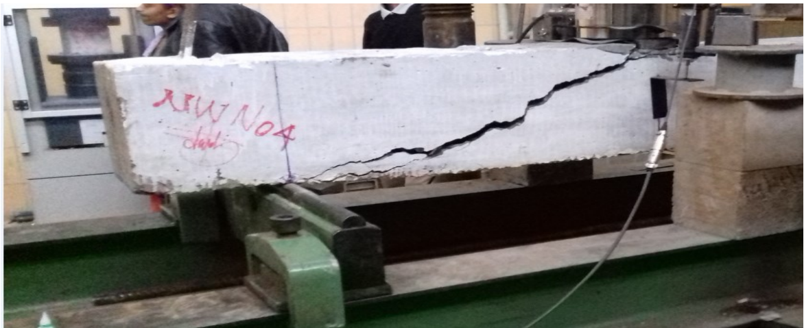
Figure 6:4: Diagonal tension failure in Specimen NWNo.4
