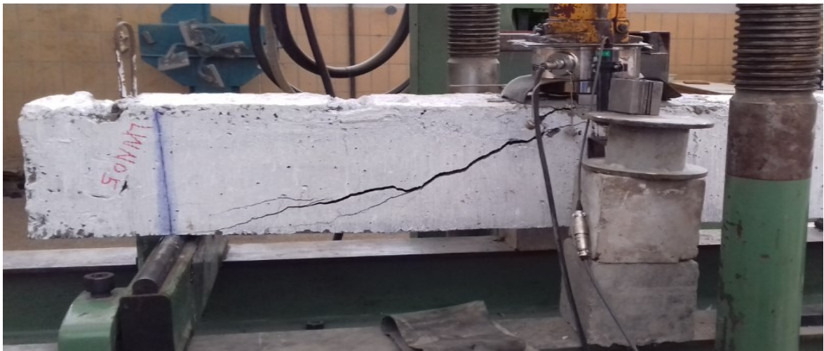
Figure 6:5: Diagonal tension failure in Specimen LWNo.5
