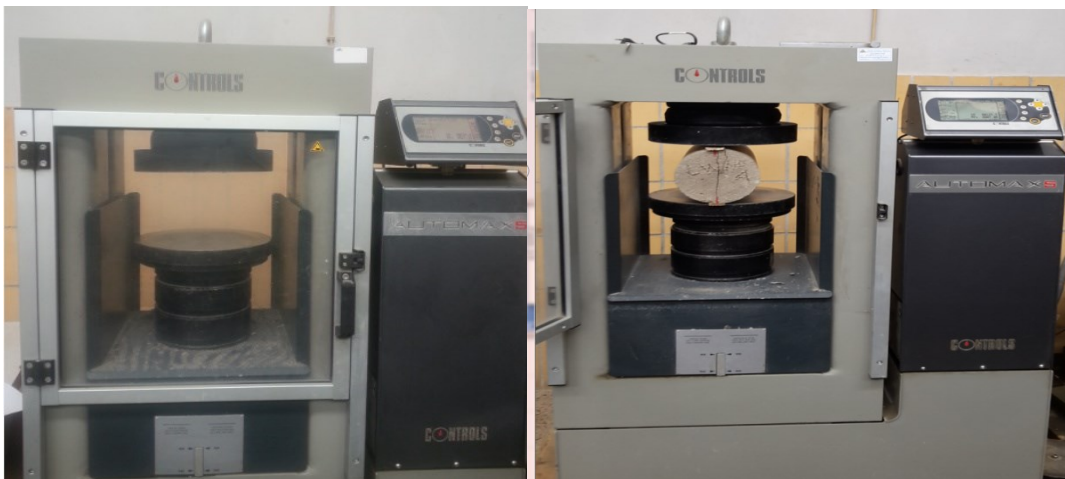
Figure 4-2 Compressive and tensile strength testing machine
