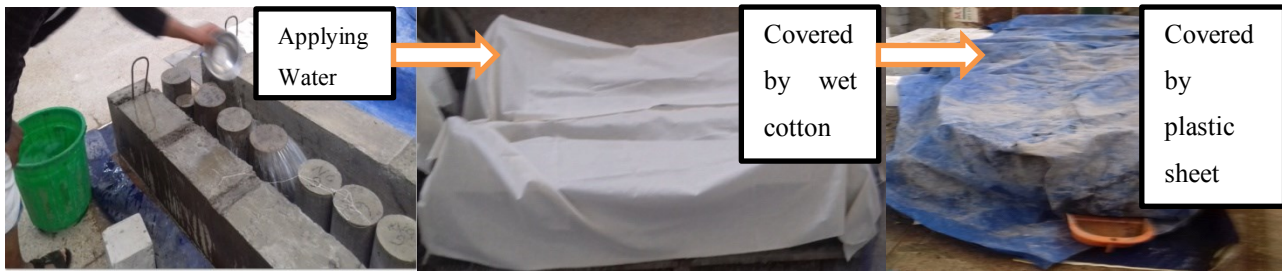
Figure 4:6: Curing process of the specimens
