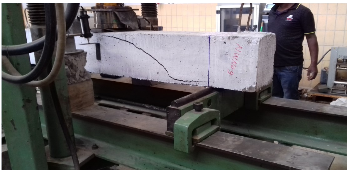
Figure 6:1: Diagonal tension failure in Specimen NWNo.9
