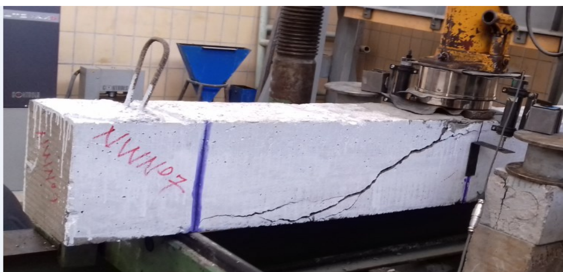
Figure 6:2: Diagonal tension failure in Specimen NWNo.7
