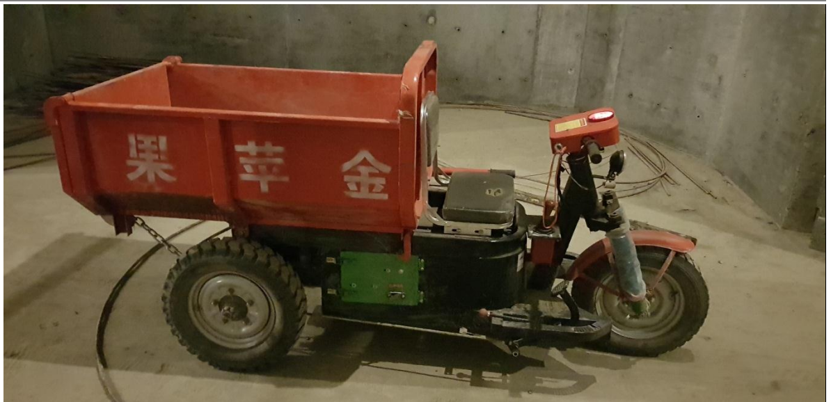
Figure 22 Damper used to transport mortar and debris
