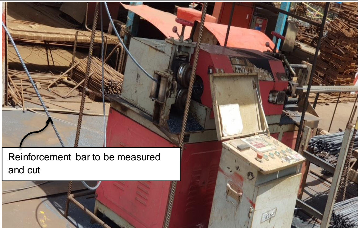
Figure 12 Reinforcement bar in roll measuring and cutting machine
