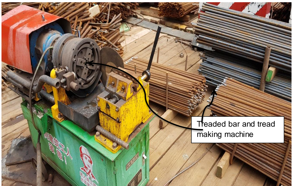
Figure 13 Reinforcement bar tread making machine
