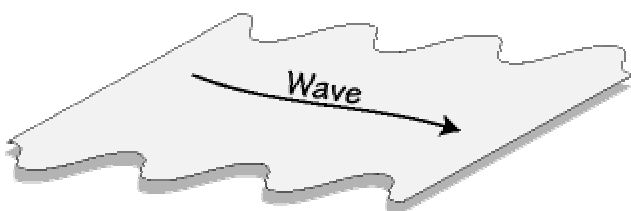
Figure 4.6 - Love wave motion (propagation)
