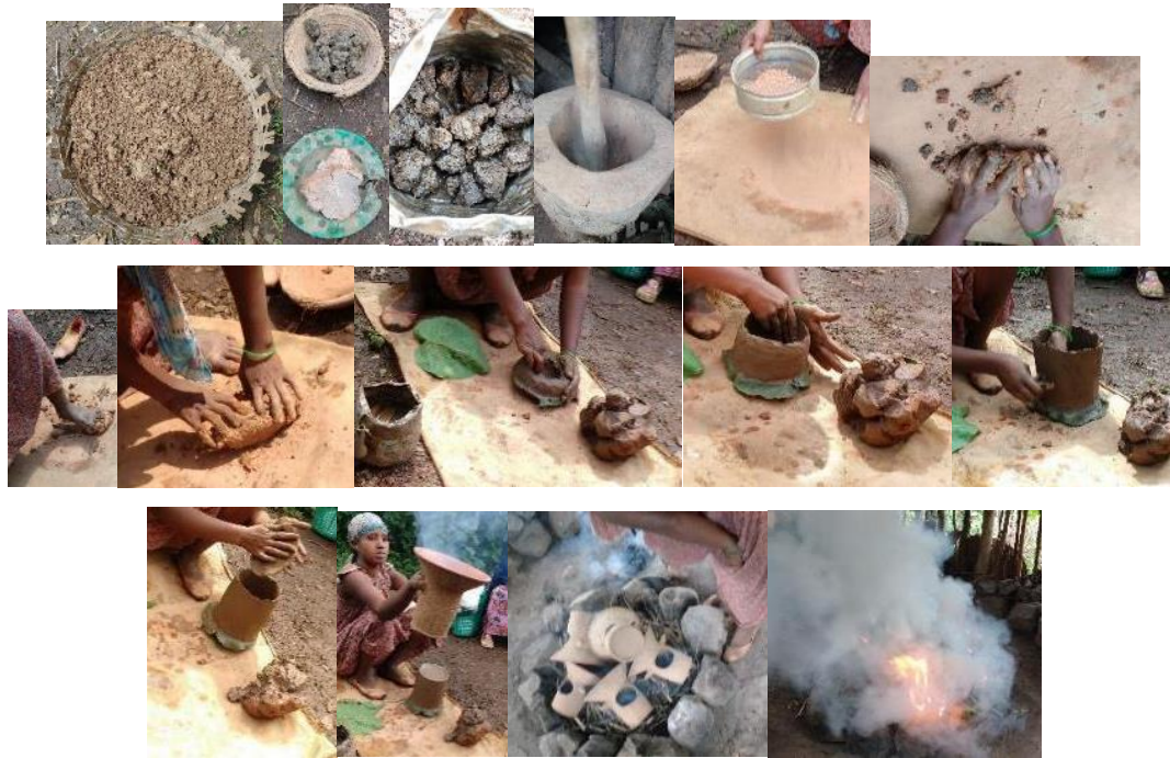
Figure 2. 10: Manufacturing process of clay pots in Ethiopia (Gondar).
