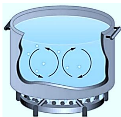
Figure 2. 1: Convection role in heat transfer inside pot of water [6].
