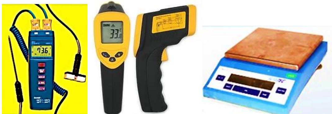
Figure 3. 3: Thermometer (contact and infrared) and mass balance,
