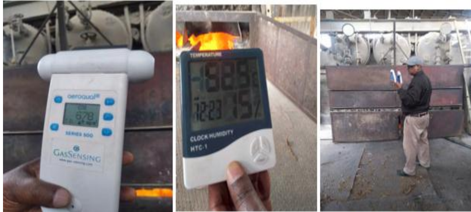
Figure 19: Air emission recording of wood log combustion
