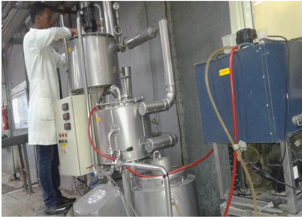
Figure 16: Micro brewery pilot plant, BGI Ethiopia plc lab.
