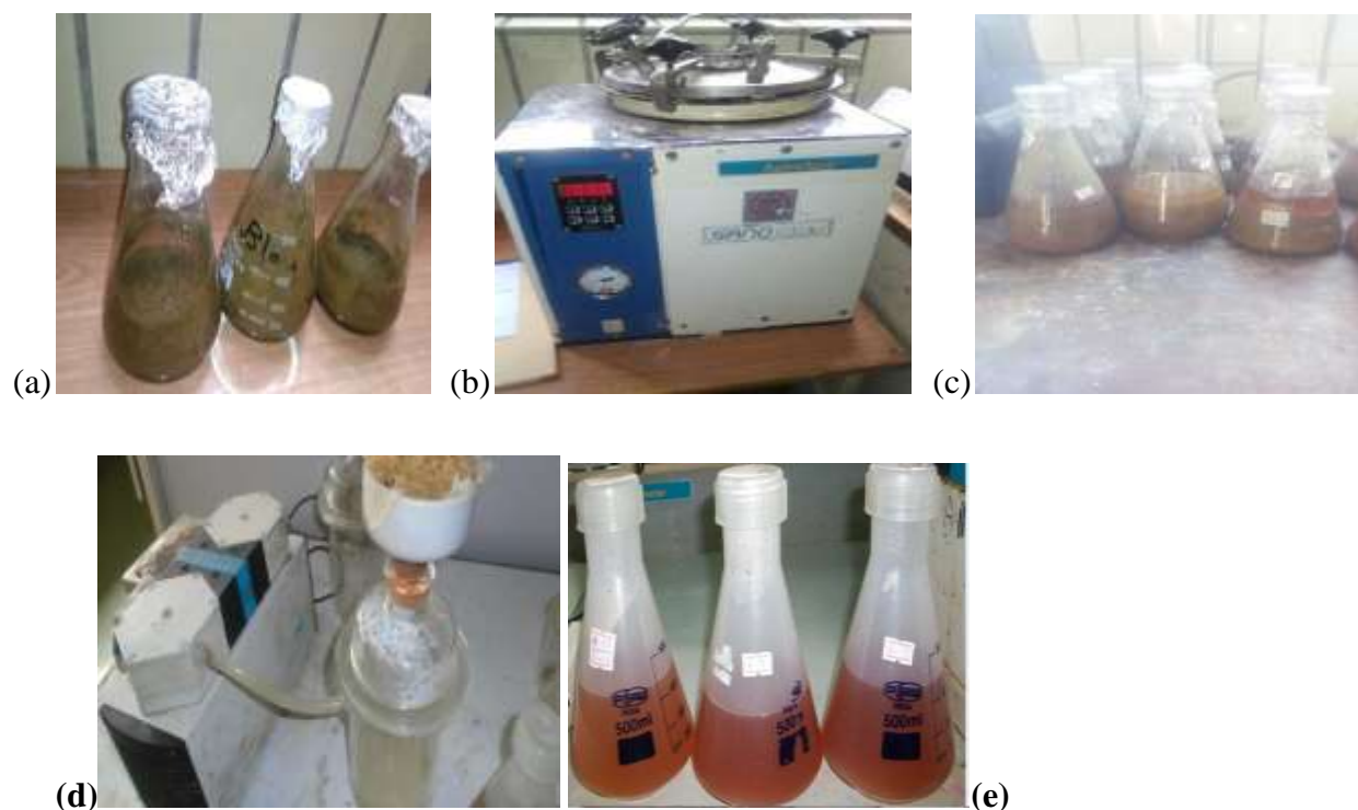
Figure 3-3: (a) Raw materials ready for pretreatment (b) Autoclave (c) Sample after pretreatment (d) Vacuum filtration, (e) Filtered sample
