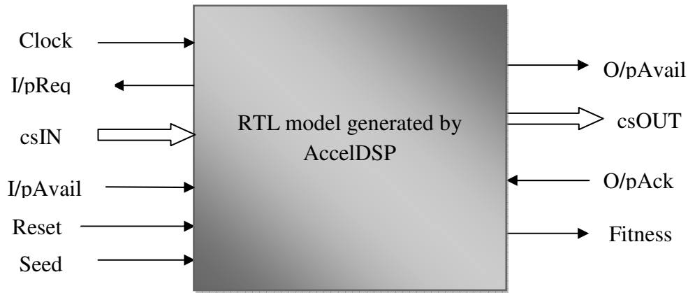
Figure 4.3 Full Handshake Interface of the hardware module
