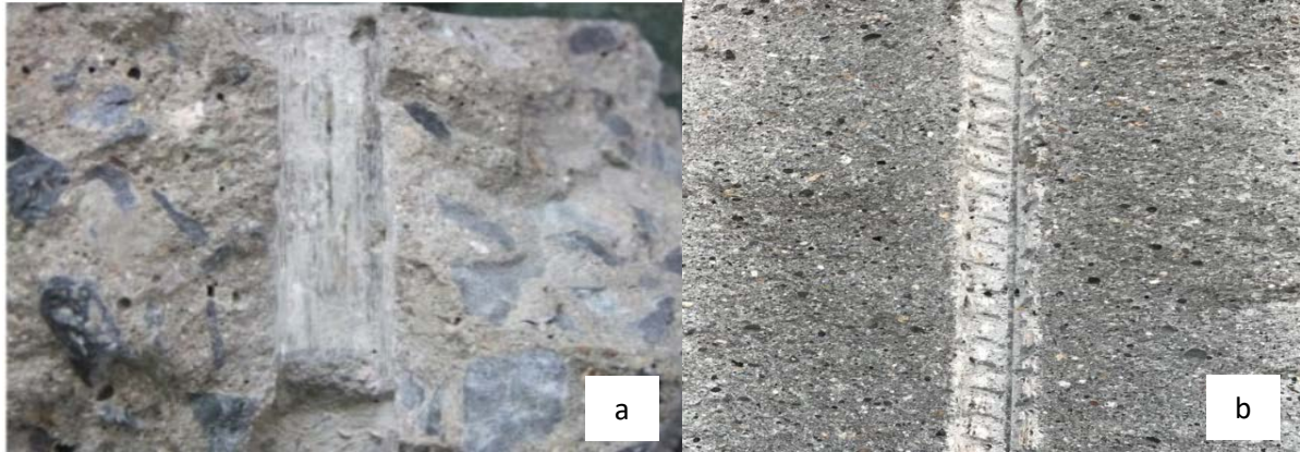
Figure 4.7. Failure patterns, Remained marks of a bar in the tested concrete specimen : (a) pull-out failure; (b) splitting failure
