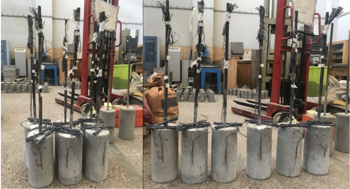
Figure 3.14. Specimen preparation for test and strain gauge arrangement
