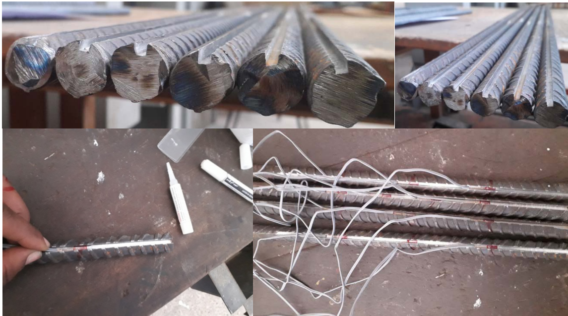
Figure 3.6. Longitudinal grooved deformed bars and application of the strain gauge on the bar
