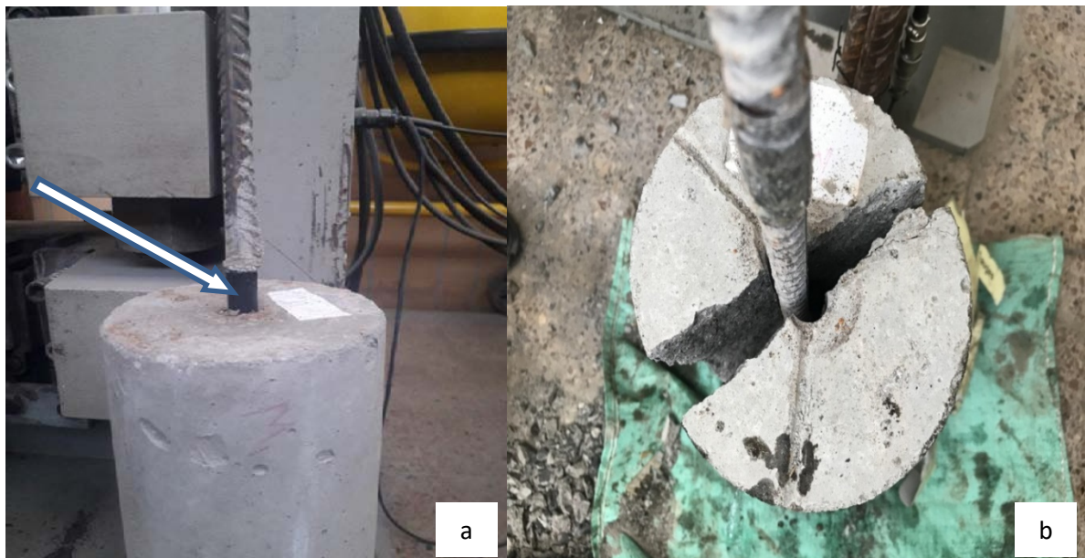
Figure 4.6. Mode of failure: (a) pull-out failure; (b) splitting failure
