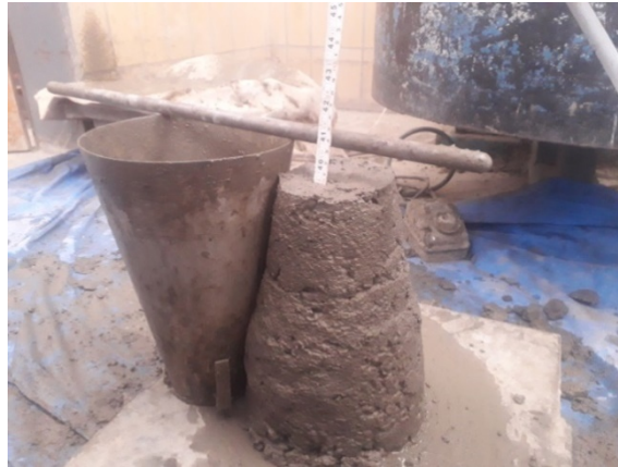
Figure 3.10. Measuring Slump of Fresh Concrete
