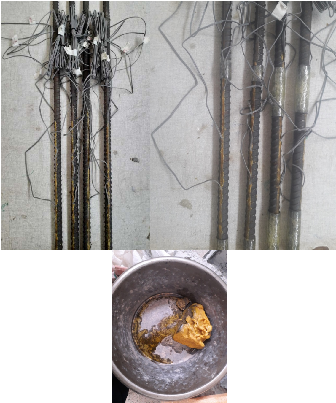
Figure 3.7. Installation of strain gauges and sealed by wax
