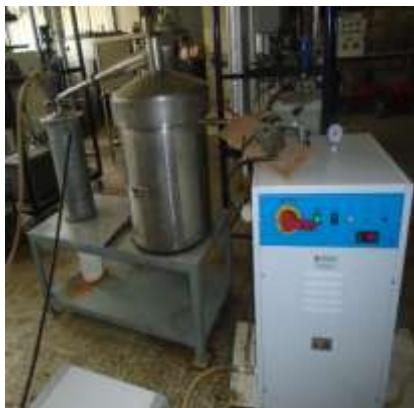
Steam distillation set up
