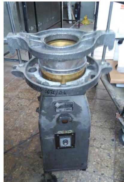
Analytical balance, sieves of different size openings with pan and mechanical shaker for determination of particle size
