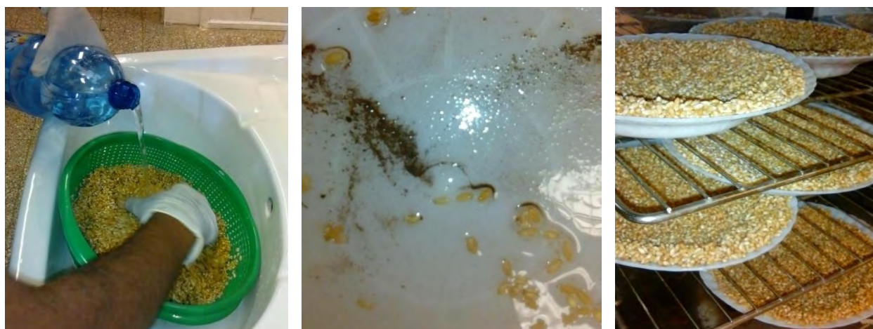
Figure 3.2. Process of washing and drying: washing the sample with deionized water in plastic bowl (left), soil residues from washed sample (center), washed samples being dried in an oven (right).
