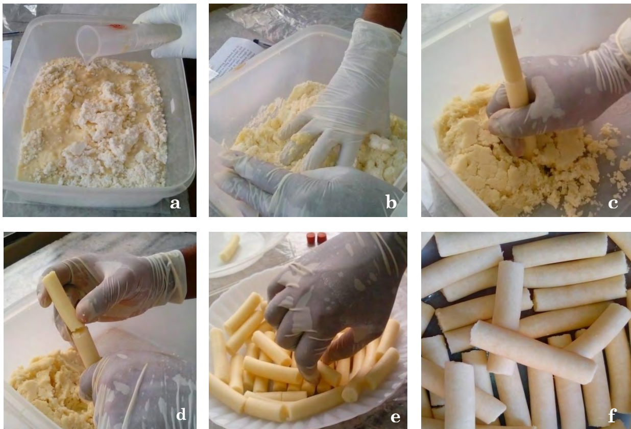
Figure 3.3: Process of making pellets: adding deionized water (a) and mixing powder diet in a plastic bowl (b), extruding the dough through a plastic tube (c), the strips cut in to shorter length pellets (d ), preparing pellets to be dried in an oven (e) and dried pellets (f).
