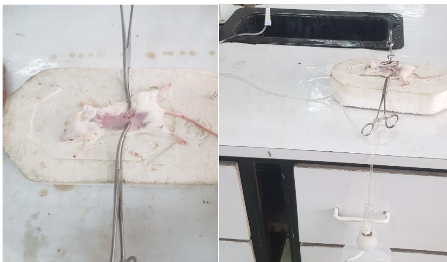
Figure 4: Water flow technique for measurement of tensile strength
